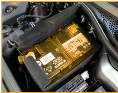
12-V Battery in Engine Compartment
