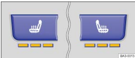
Fig. 47 In the center console: Seat heating buttons for the front seats.
