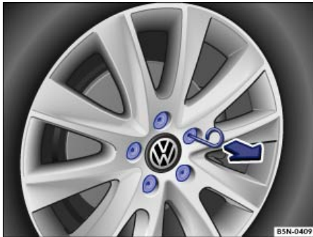
Fig. 177 Pulling cover caps off wheel bolts.
