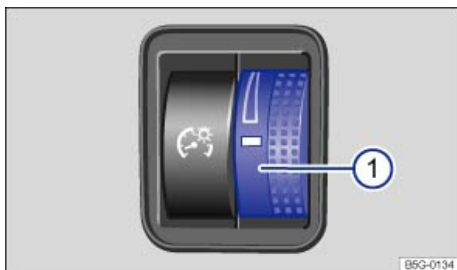
Fig. 78 To the left of the steering wheel: Thumbwheel to adjust instrument panel lighting 1.
