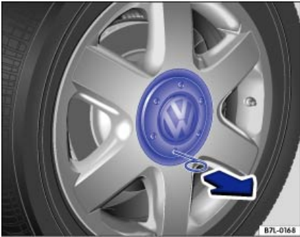
Fig. 175 Pulling the hubcap off.
