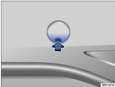
Fig. 192 In the right rear bumper: Removing the cover.
