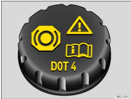
Fig. 135 In the engine compartment: Brake fluid reservoir cap (cap design may vary depending on vehicle equipment).
