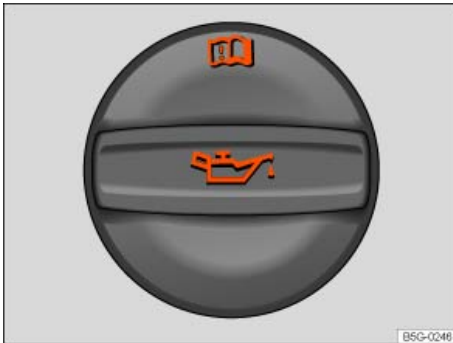
Fig. 157 In the engine compartment: Engine oil filler cap.
