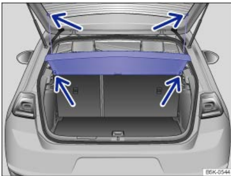
Fig. 91 In the luggage compartment: Installing and removing the luggage compartment cover.
