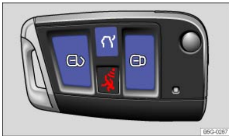
Fig. 23 Remote control vehicle key with panic button.
