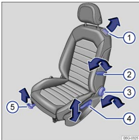
Fig. 36 Driver seat: Manual seat adjustment controls.
