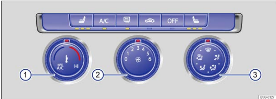
Fig. 149 In the center console: Manual air conditioning controls.
