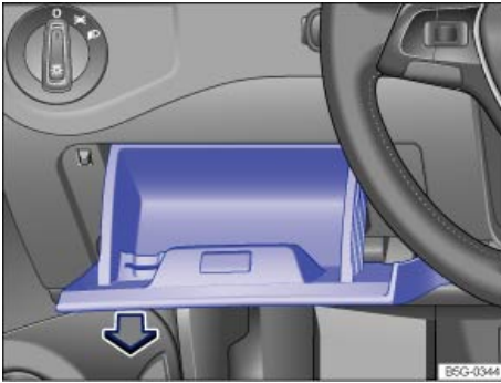
Fig. 184 On the driver side in the instrument panel: Fuse box cover.
