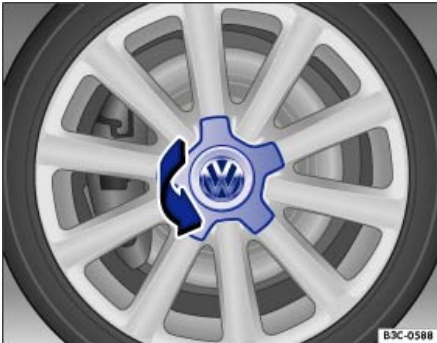
Fig. 176 Twisting the hubcap off.
