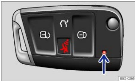
Fig. 20 Indicator light in the remote control vehicle key.
