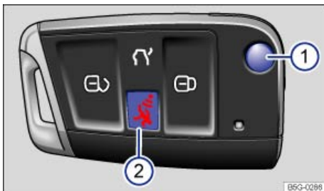
Fig. 19 Remote control vehicle key with panic button.
