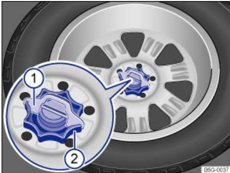
Fig. 105 In the luggage compartment: Handwheel holding the spare wheel in place.
