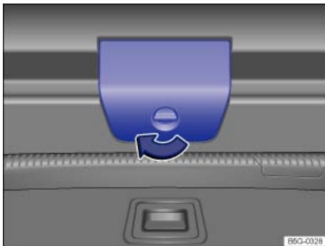
Fig. 169 Inside the luggage compartment: Cover for the rear hatch release.
