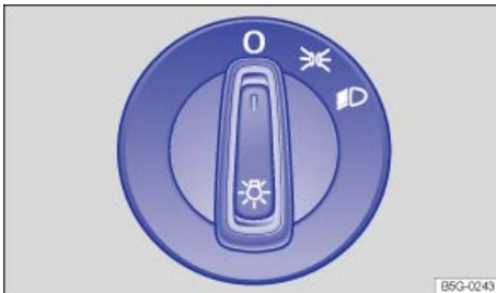
Fig. 76 Headlight switch next to the steering wheel.
