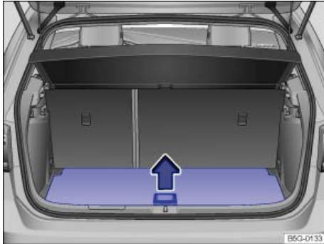
Fig. 96 In the luggage compartment: Opening the variable luggage compartment floor.
