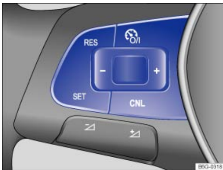
Fig. 140 Left-hand side of the multi-function steering wheel (if equipped): Buttons for operating the cruise control .
