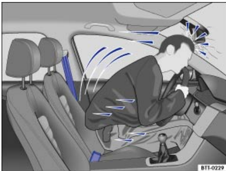
Fig. 51 The unbelted driver is thrown forward.
