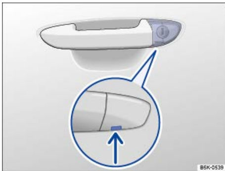
Fig. 166 Door handle on driver door: Concealed lock cylinder (if applicable).
