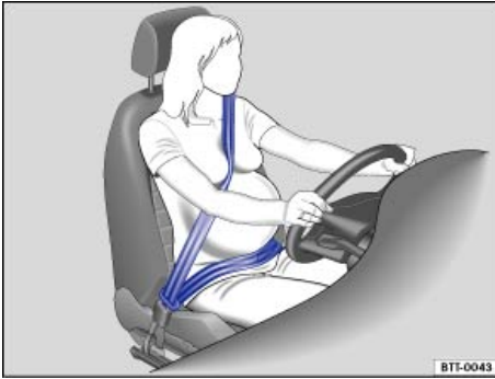
Fig. 57 Proper safety belt positioning for expectant mothers.
