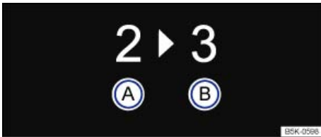
Fig. 133 In the instrument cluster display: Gear recommendation.
