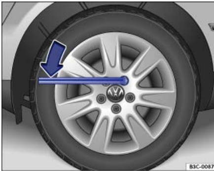
Fig. 179 Changing a wheel: Loosening the wheel bolts.
