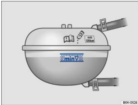
Fig. 159 Coolant expansion tank in the engine compartment.
