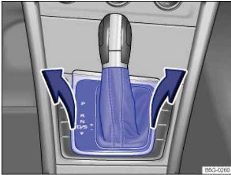
Fig. 171 Removing the selector gate cover.
