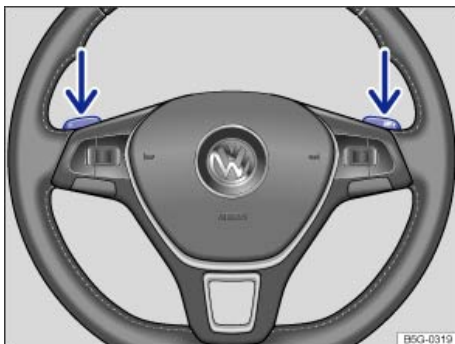
Fig. 132 Steering wheel with Tiptronic shift paddles (if equipped).
