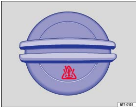
Fig. 160 Coolant expansion tank cap in the engine compartment.
