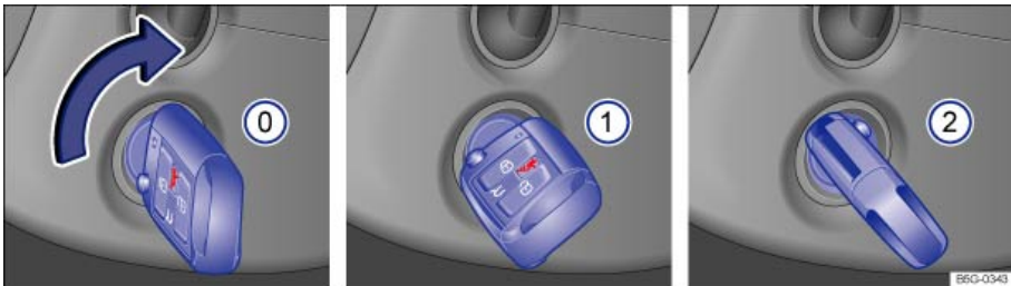
Fig. 123 In the ignition switch: Vehicle key positions.
