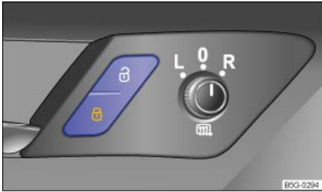
Fig. 24 In the driver and passenger doors: Power locking button.
