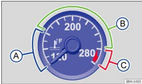
Fig. 158 Engine coolant temperature gauge in the instrument cluster: A Engine cold; B Normal temperature range; C Warning zone.
