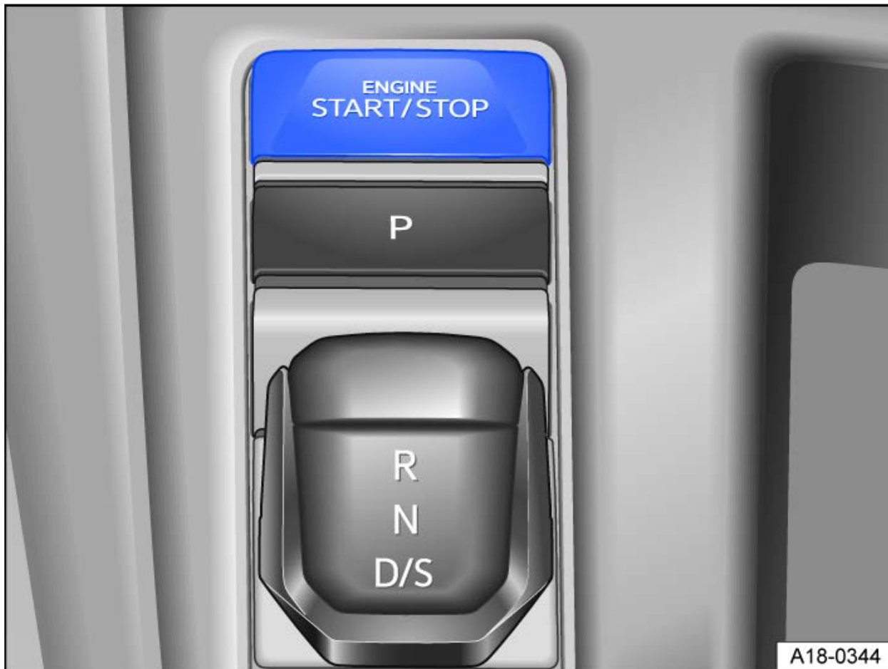
Fig. 2 Located in the lower area of the center console: Starter button for starting the engine (in vehicles with a DSG® automated transmission).
