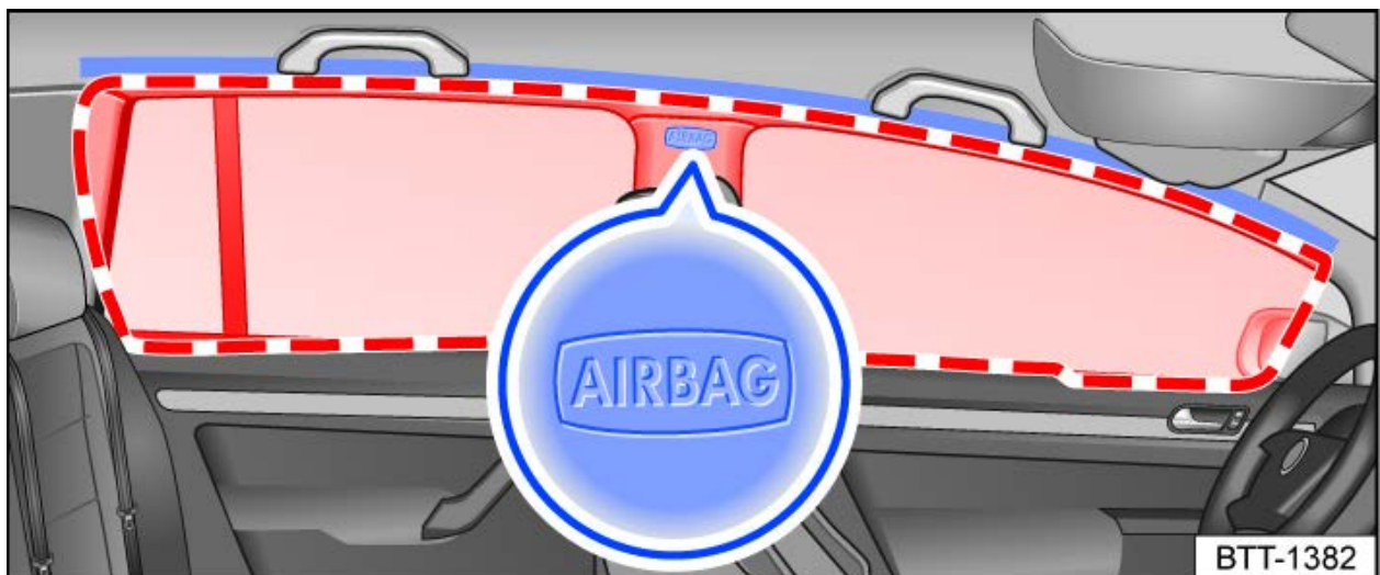
Fig. 1 On the left side of the vehicle: location and deployment zone of the Side Curtain Protection®.
