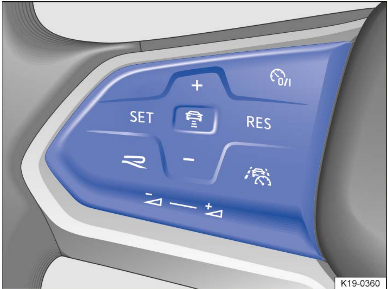
Fig. 1 Left side of the multi-function steering wheel: buttons for Travel Assist operation.
