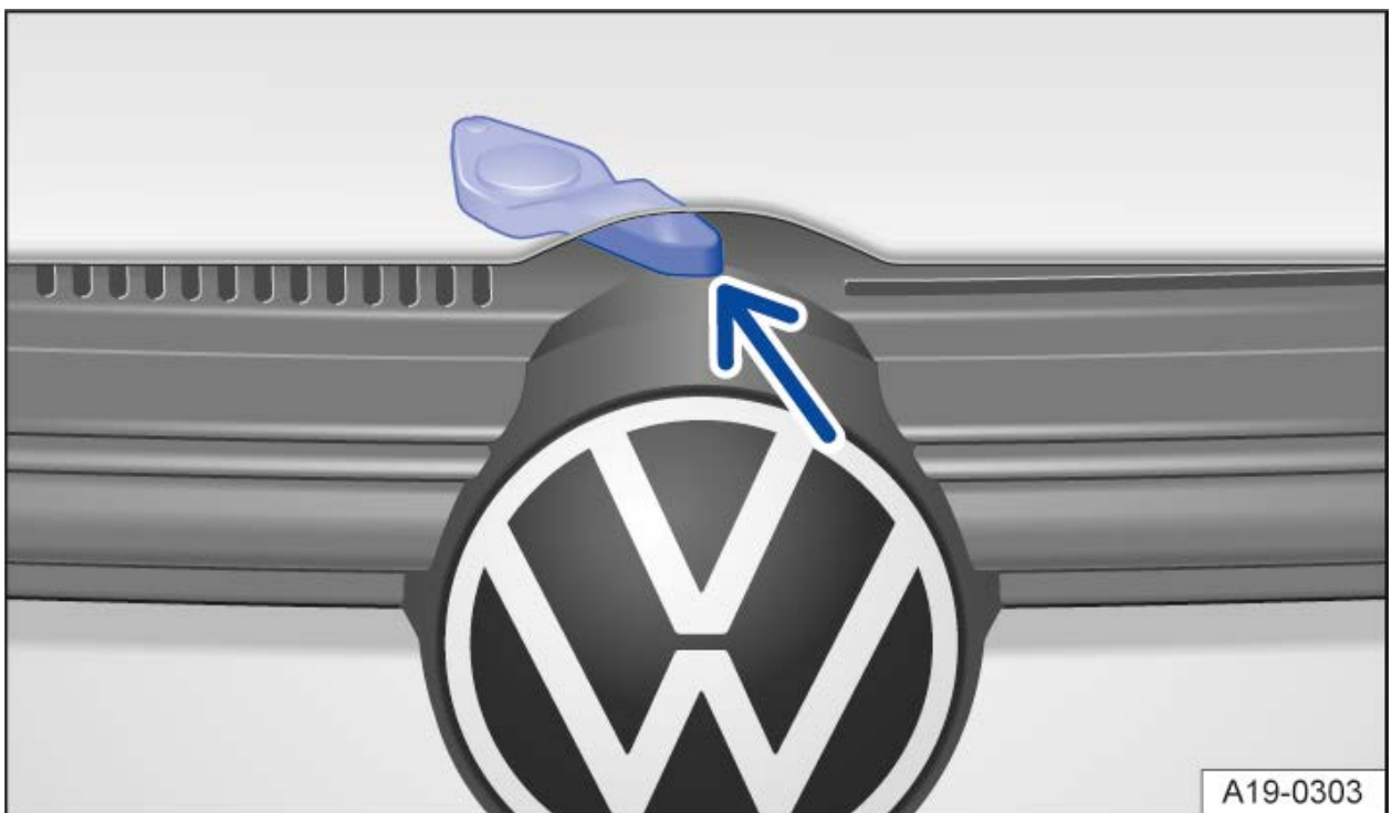
Fig. 2 Above the radiator grille: Opening lever for the hood.
