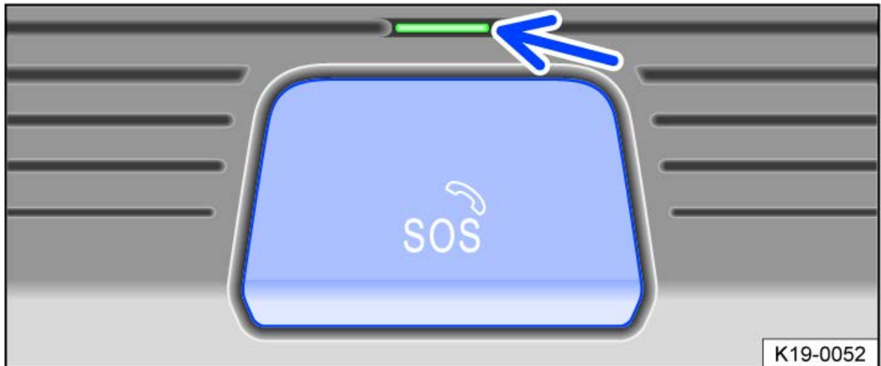
Fig. 2 In the overhead console: control for the Emergency Call Service (behind the cover over the button).
