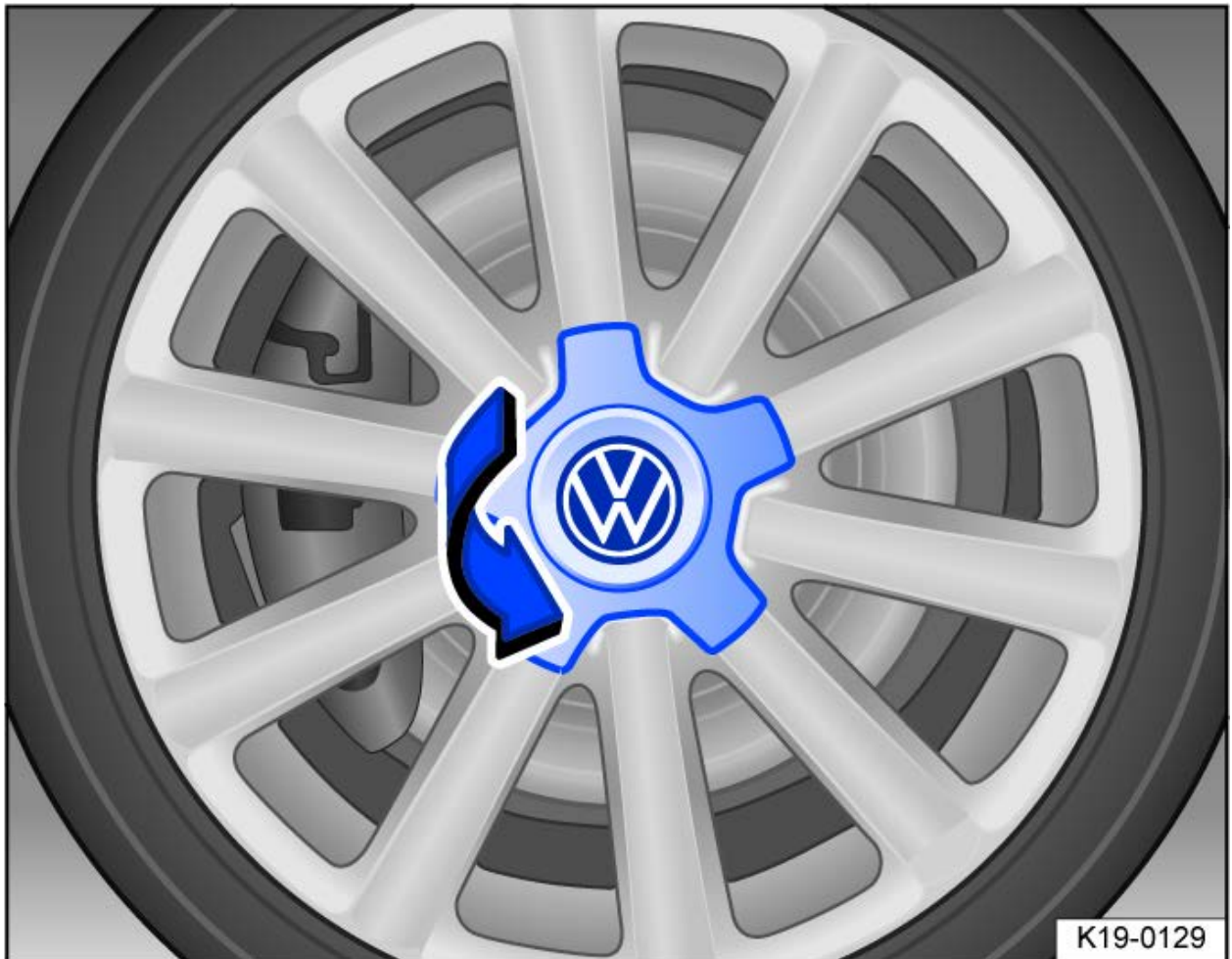
Fig. 2 Twist off the hubcap.
