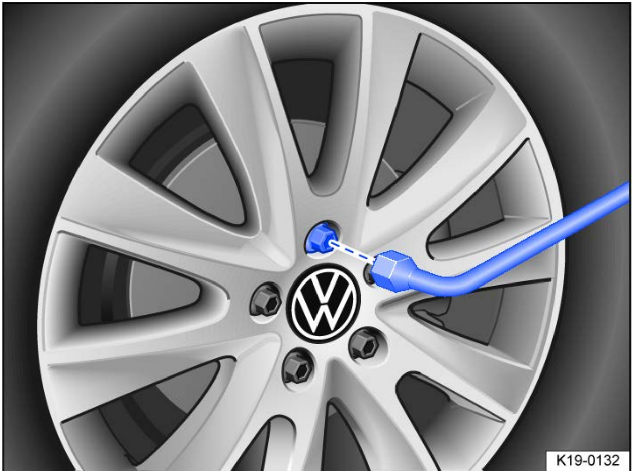
Fig. 1 Wheel change: removing wheel bolts with the screwdriver handle.
