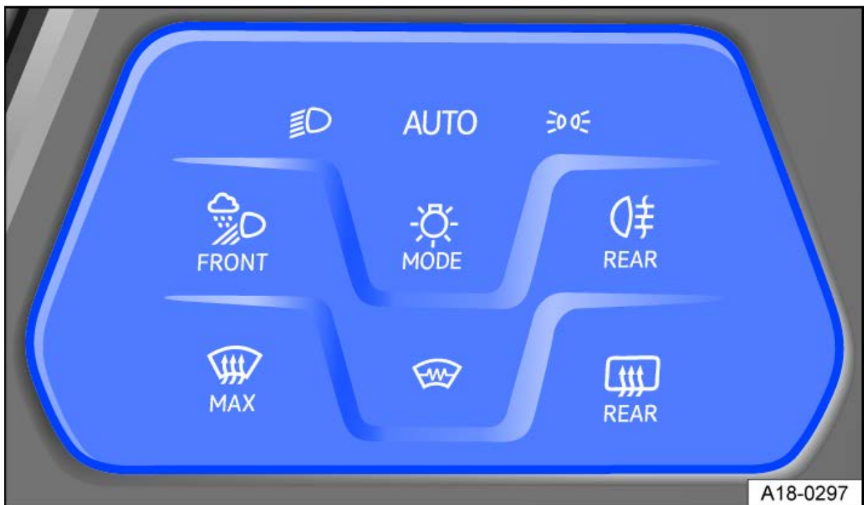
Fig. 1 Next to the steering wheel: Button to switch on the exterior lighting.
