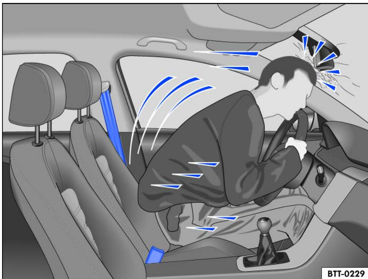
Fig. 1 A driver not wearing a safety belt is propelled forward.
