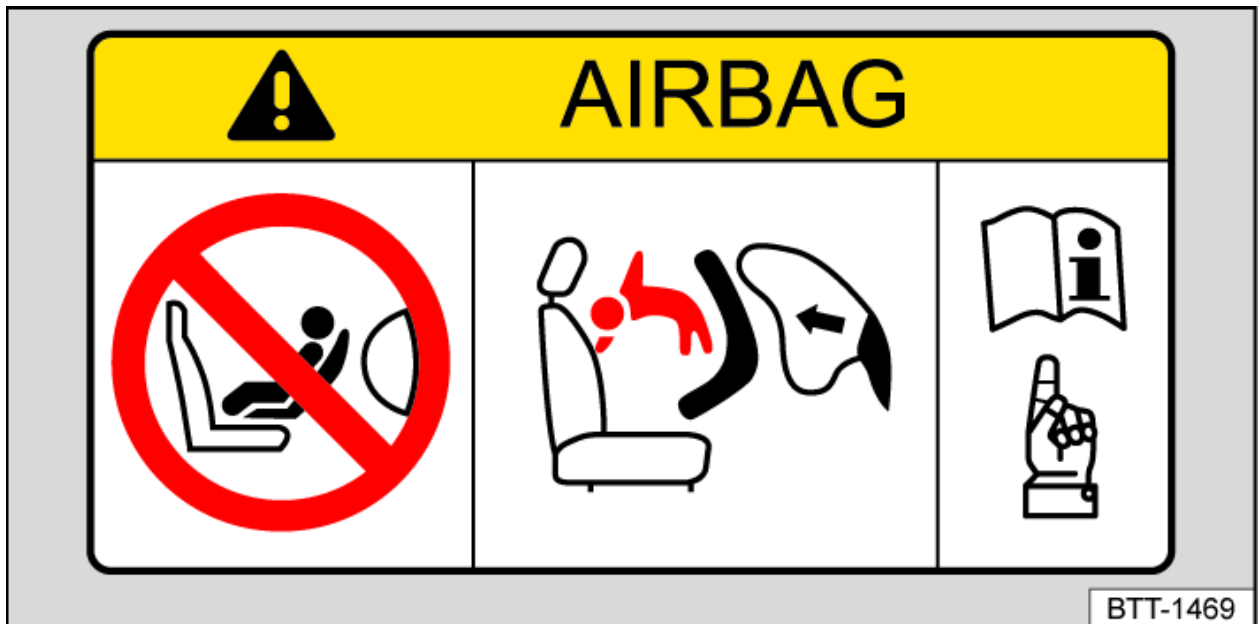
Fig. 1 General example: airbag label on the sun visor.
