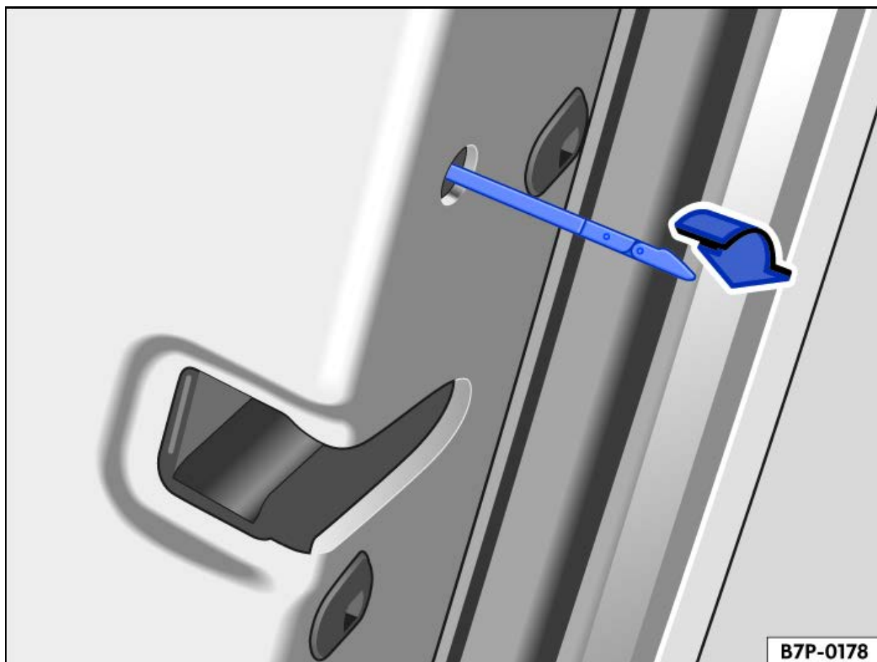
Fig. 1 In the front edge of the rear right-hand door: Vehicle emergency unlock for using the spare (mechanical) key.
