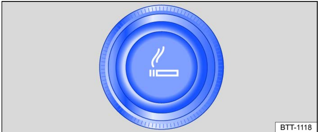
Fig. 1 In the lower section of the center console: Cigarette lighter.
