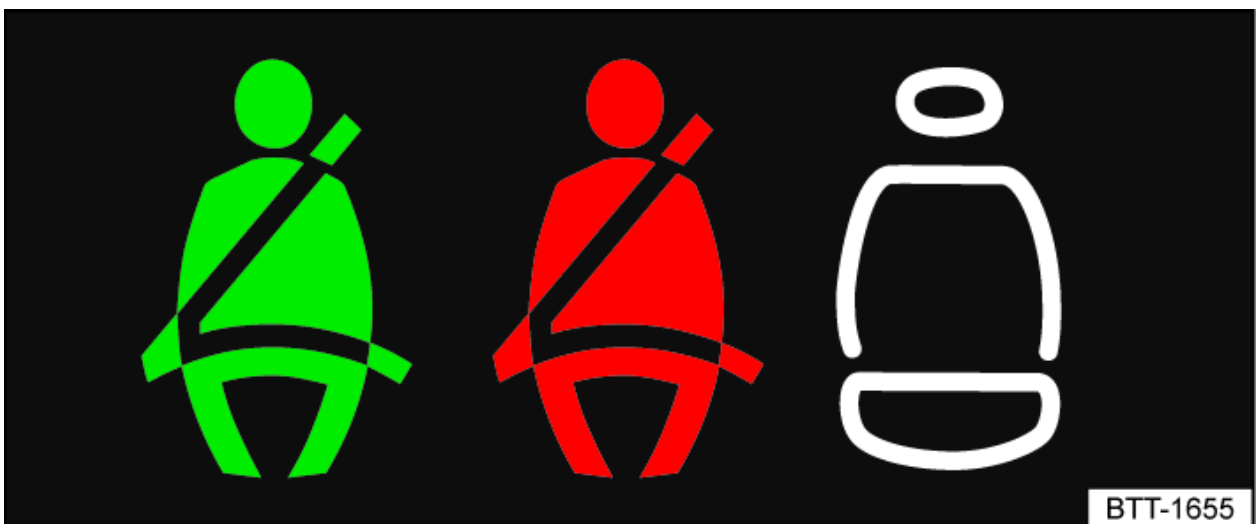
Fig. 2 In the instrument cluster display: safety belt status indicator for the rear seats.
