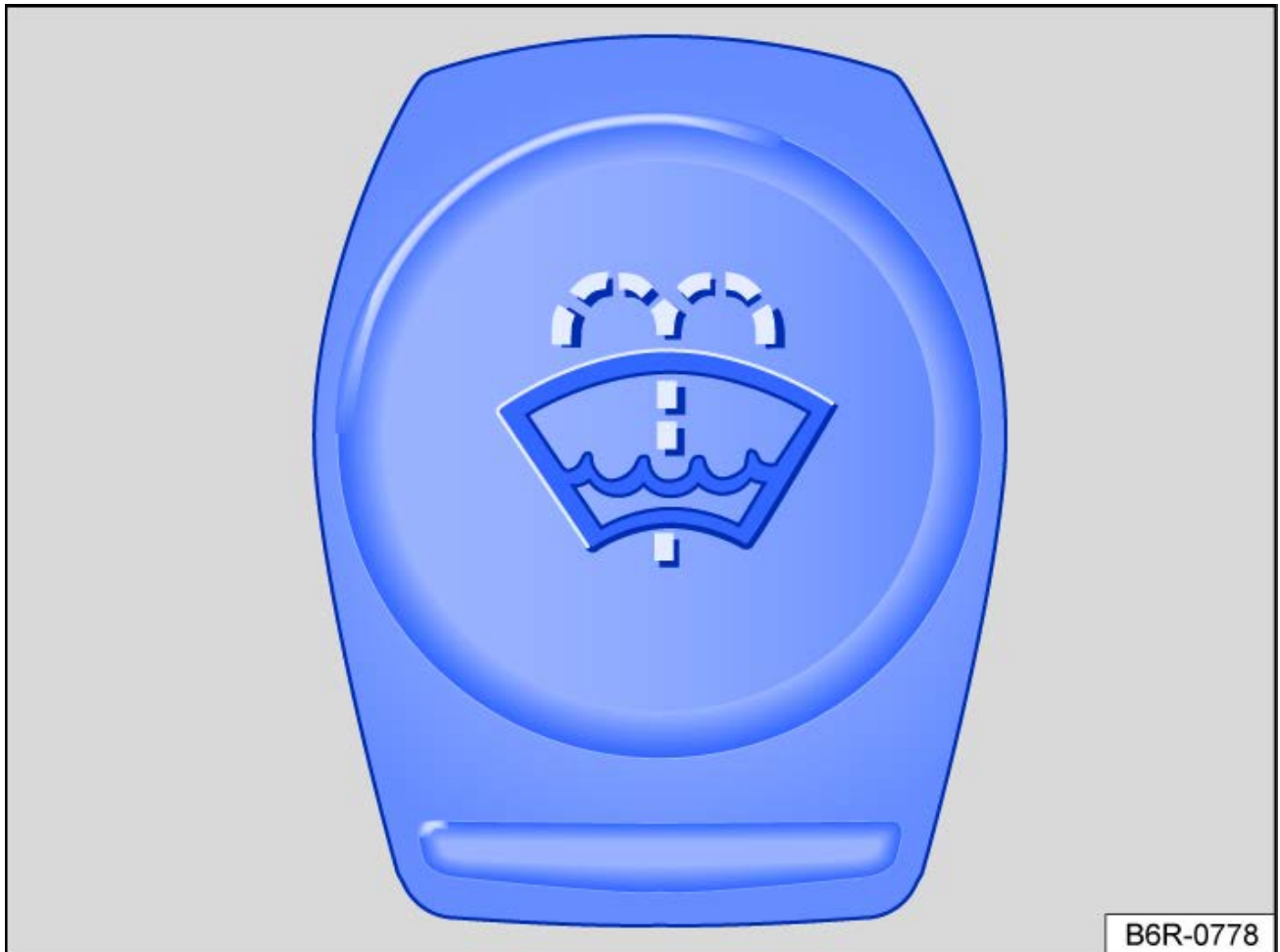
Fig. 1 In the engine compartment: cap on the washer fluid reservoir.
