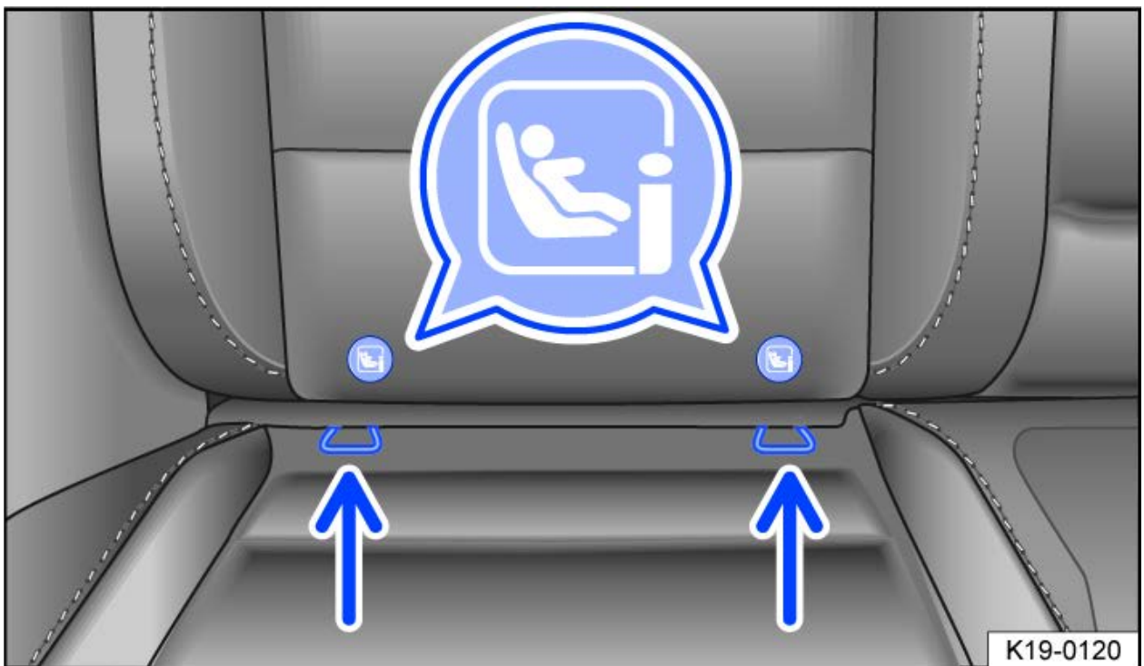
Fig. 2 Designation of the i-Size anchor points for child restraints.
