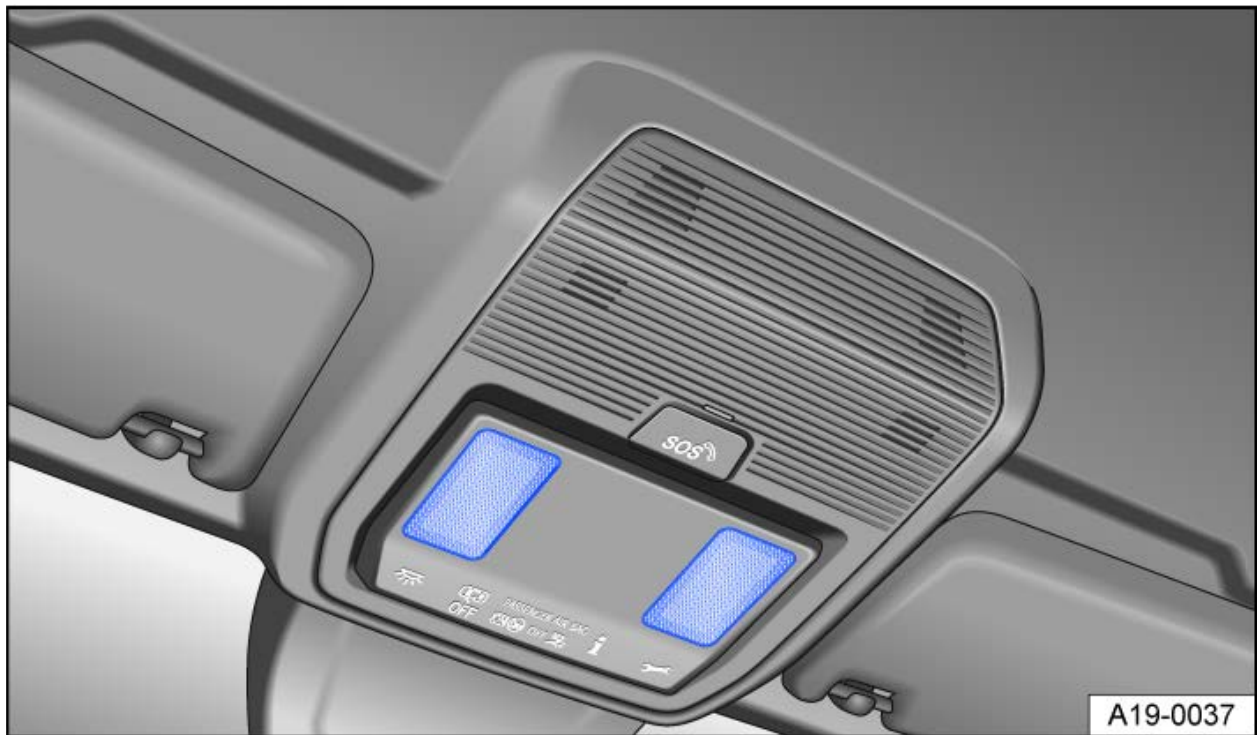
Fig. 1 On the overhead console: touch-sensitive reading lights.
