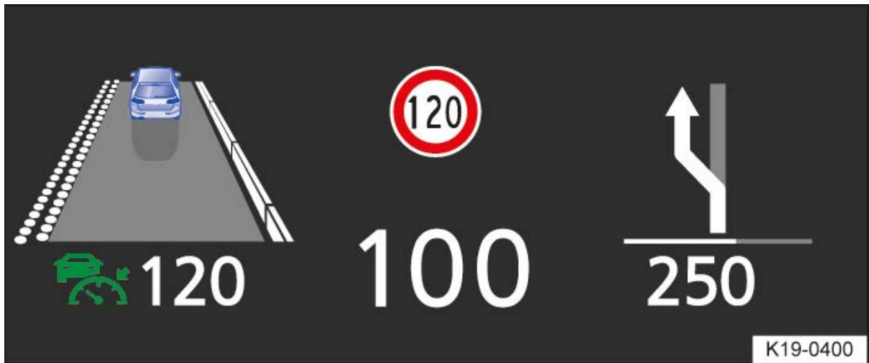
Fig. 1 In the visual range of drivers: sample displays on the head-up display
