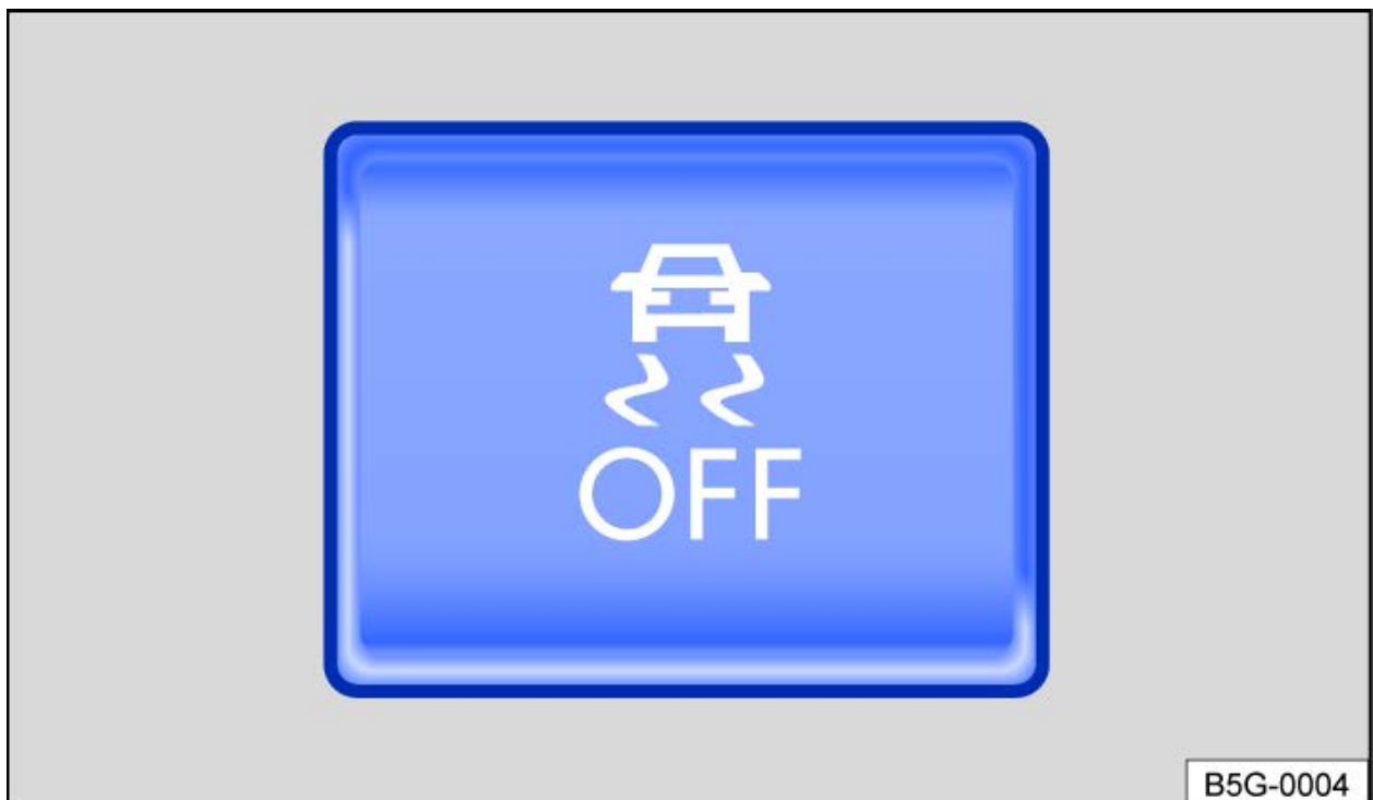
Fig. 1 In the center console: Button to manually switch off and on ASR, ESC or ESC Sport (depending on vehicle equipment).
