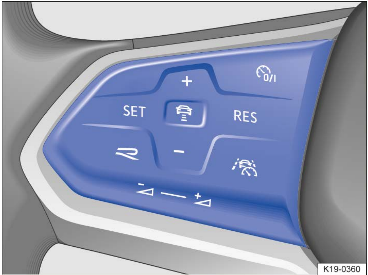
Fig. 2 Left side of the multi-function steering wheel: buttons for cruise control system operation (option 2).
