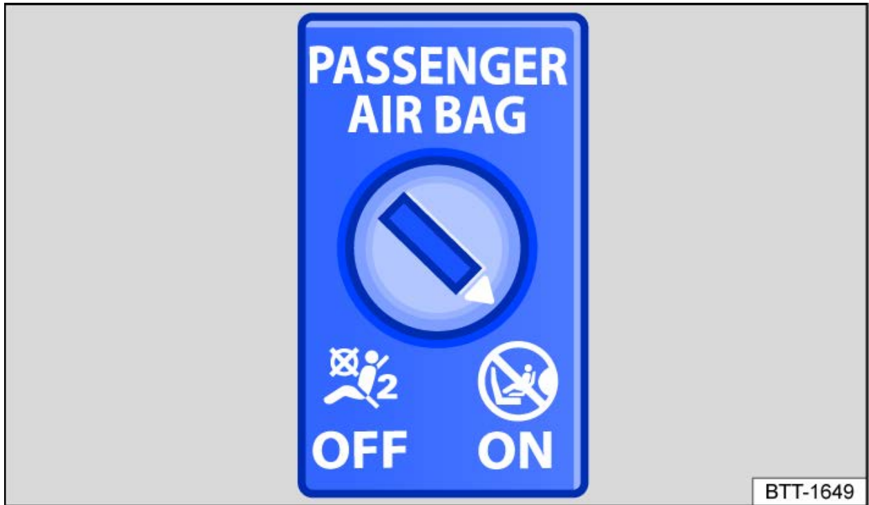
Fig. 1 In the instrument panel on the front passenger side: Key-operated switch to turn on and off the front passenger airbags.
