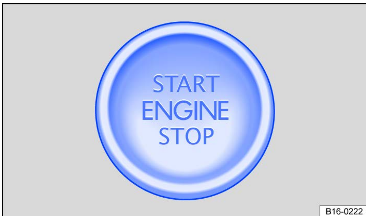
Fig. 1 Located in the lower area of the center console: Starter button for starting the engine (in vehicles with a manual gearbox).
