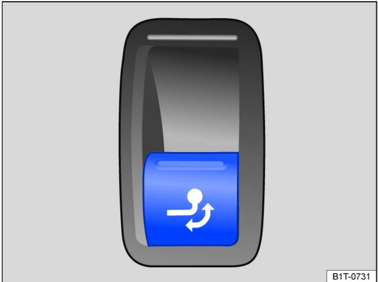
Fig. 1 On the right side of the luggage compartment: button for releasing the ball head.
