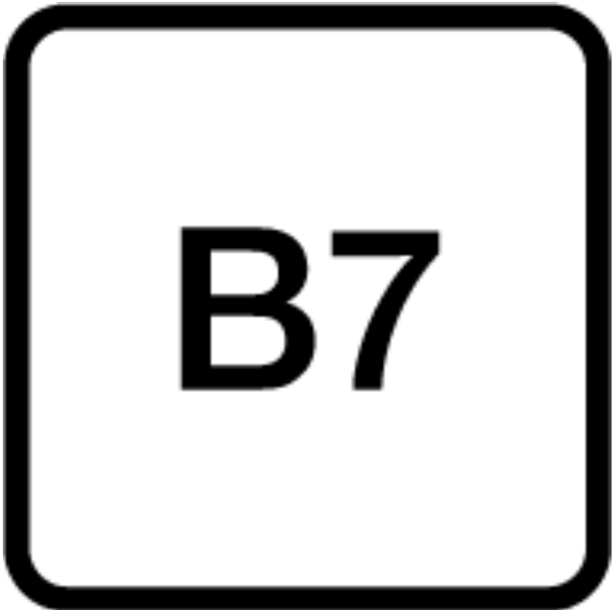
Fig. 3 Diesel fuel containing biodiesel
