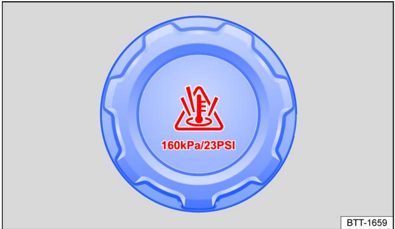
Fig. 2 In the engine compartment: cap on the engine coolant expansion tank.
