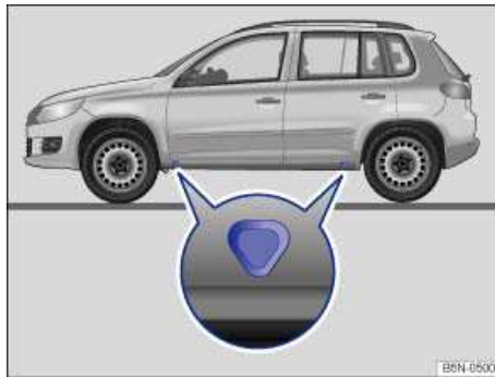
Fig. 196 Lift points for the jack.
