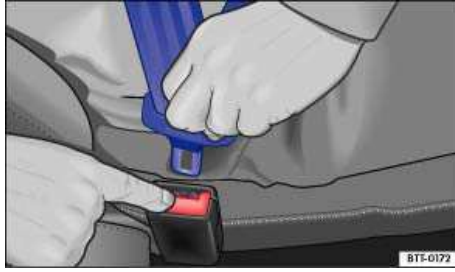
Fig. 66 Releasing the buckle tongue from the belt buckle.
