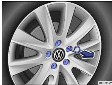
Fig. 193 Pulling cover caps off wheel bolts.
