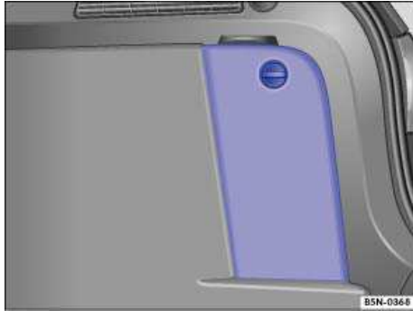
Fig. 130 On the right in the luggage compartment: Side storage compartment.
