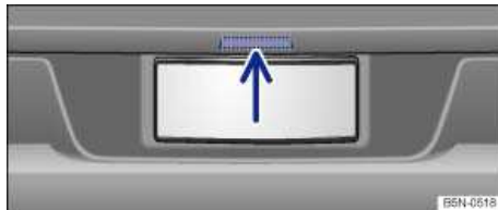
Fig. 34 Opening rear hatch from the outside.
