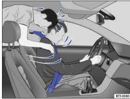
Fig. 63 Unbelted passengers in the rear seats are thrown forward on top of the belted driver.
