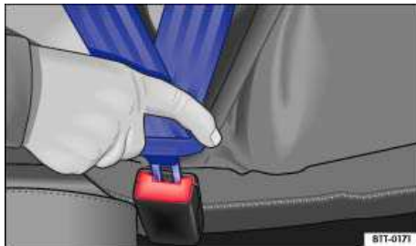
Fig. 65 Inserting the buckle tongue into the belt buckle.
