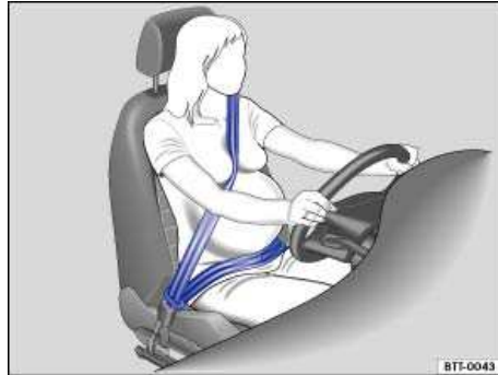
Fig. 68 Proper safety belt positioning for expectant mothers.
