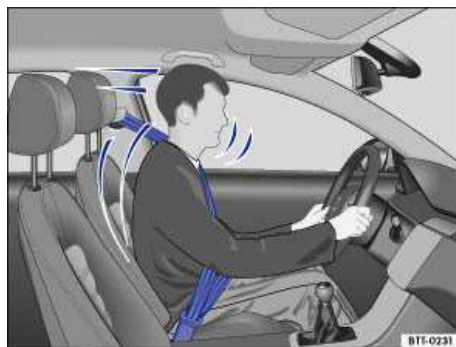
Fig. 64 Belted driver secured by the correctly worn safety belt in the event of a sudden braking maneuver.
