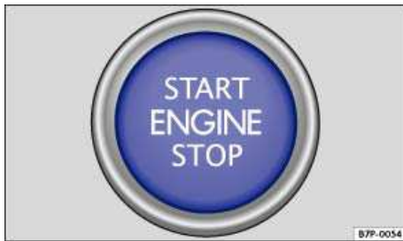
Fig. 136 In the center console: Starter button of the Keyless Access with push button start.
