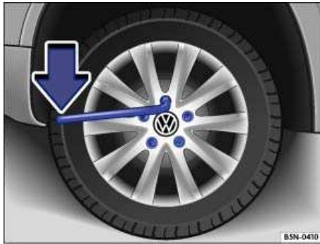
Fig. 195 Changing a wheel: Loosening wheel bolts.
