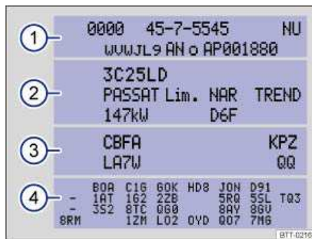
Fig. 20 Vehicle identification label: Shown in the example with engine identification code CBFA 3.
