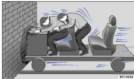
Fig. 61 A vehicle with passengers not wearing safety belts hits a wall.
