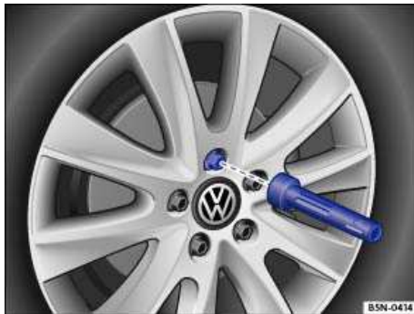
Fig. 198 Changing a wheel: Remove previously loosened wheel bolts using the screwdriver handle.
