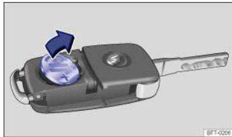
Fig. 26 Remote control vehicle key: Remove old battery.
