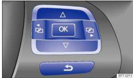
Fig. 17 Premium version (vehicles with menu control multi-function steering wheel): Buttons on the right side of the steering wheel.
