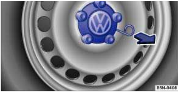
Fig. 271 Removing the centre covers by pulling.
