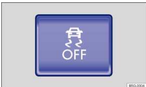
Fig. 195 In the lower part of the centre console: button for switching traction control system, traction control system with Electronic Stability Control or ESC Sport on and off manually.
