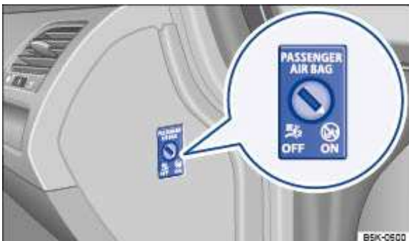
Fig. 17 In the dash panel on the front passenger side: key-operated switch for switching the front passenger front airbag on and off.
