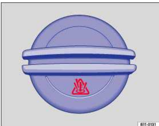
Fig. 260 In the engine compartment: coolant expansion tank cap.
