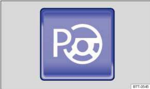
Fig. 187 In the lower section of the centre console: button for switching on Park Assist.
