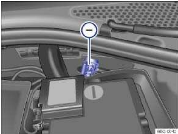
Fig. 246 In the engine compartment: jump start connection point (earth connection).
