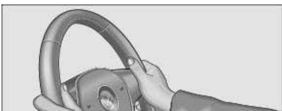
Fig. 64 Below the steering wheel in the steering column trim: lever for mechanical adjustment of the steering wheel position.
