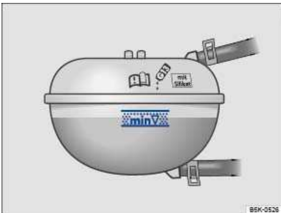
Fig. 259 In the engine compartment: markings on the coolant expansion tank.
