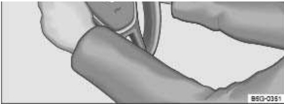
Fig. 65 On the steering wheel: 9 o'clock and 3 o'clock position.
