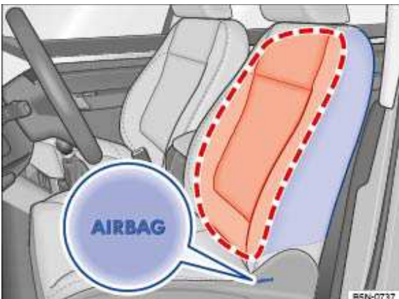
Fig. 19 On the side of the front seat: location and deployment zone of the side airbag.
