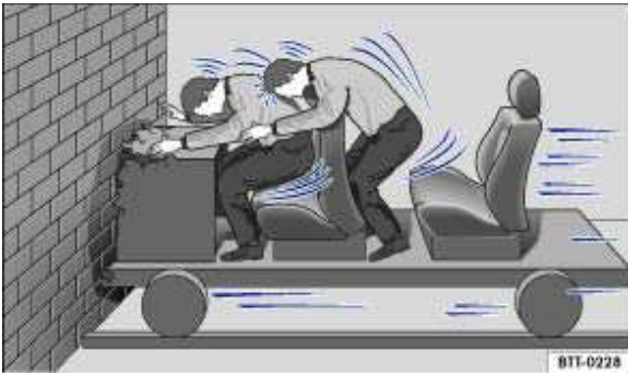
Fig. 5 Unbelted occupants in a vehicle striking a brick wall.
