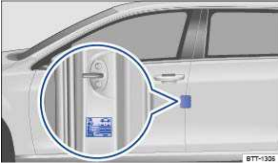
Fig. 267 On the driver door pillar: tyre pressure sticker (alternatively on the inside of the fuel flap).
