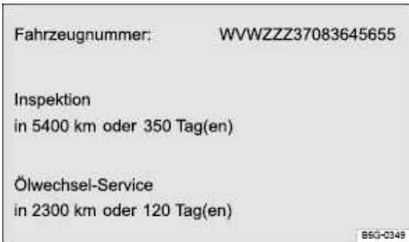
Fig. 57 Infotainment system screen: example of a display containing service information screen (illustration).
