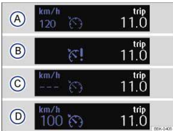
Fig. 151 Instrument cluster display: cruise control system status display.
