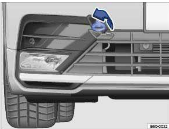
Fig. 251 Front bumper, right-hand side: screwing in the towing eye.
