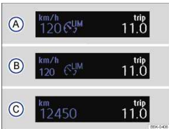
Fig. 154 On the instrument cluster display: speed limiter status displays.
