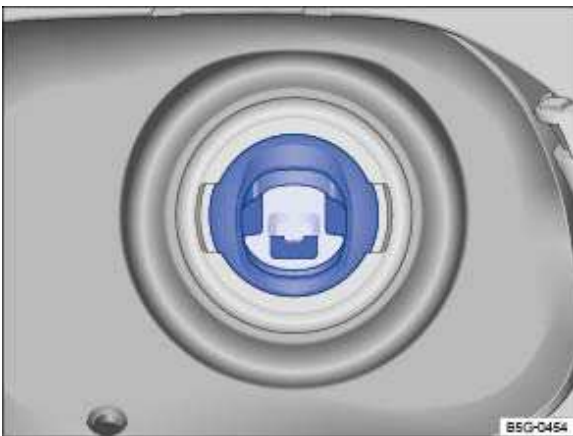
Fig. 229 Illustration: misfuelling prevention device in the tank filler neck.
