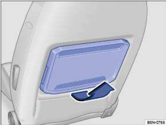
Fig. 105 Front seat: setting up the folding table.
