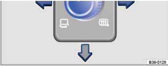
Fig. 117 In the driver door: rotary knob for the exterior mirrors.
