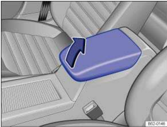
Fig. 200 Between the front seats: stowage compartment in the front centre armrest.
