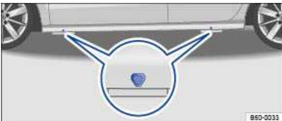
Fig. 276 Lifting points for the jack.
