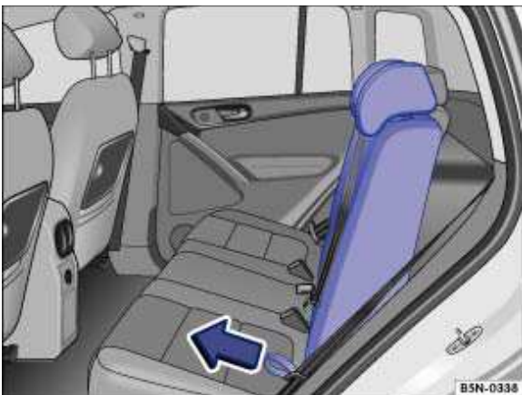
Fig. 96 Folding the backrest forwards and backwards.
