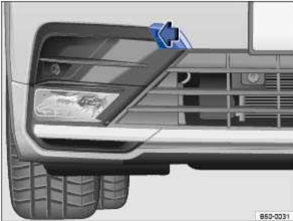
Fig. 250 In the right-hand side of the front bumper: cover for the towing eye mounting.
