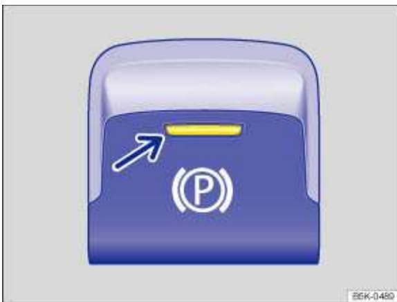
Fig. 173 In lower part of centre console: button for the electronic parking brake.
