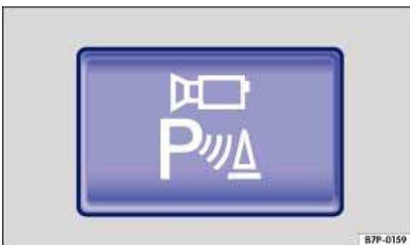
Fig. 191 In the upper part of the centre console: button for switching on the Area View.
