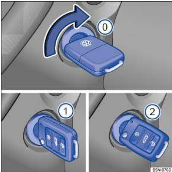
Fig. 133 To the right of the steering wheel: positions of the vehicle key in the ignition lock.
