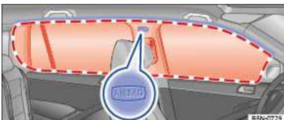
Fig. 20 On the left-hand side of the vehicle: location and deployment zone of the curtain airbag.
