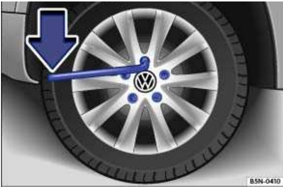
Fig. 274 Changing a wheel: loosening the wheel bolts.
