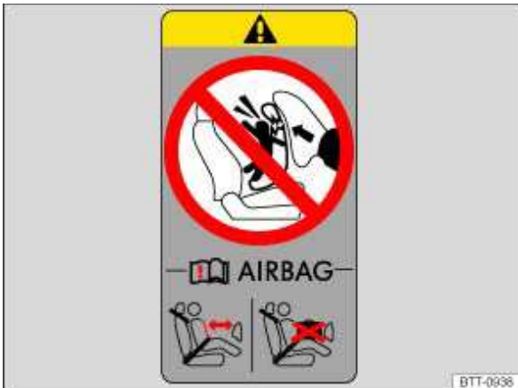
Fig. 25 A typical airbag label on the B-pillar.
