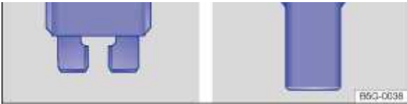
Fig. 244 Remove or insert fuse with plastic pliers: flat blade fuse, JCASE® fuse.
