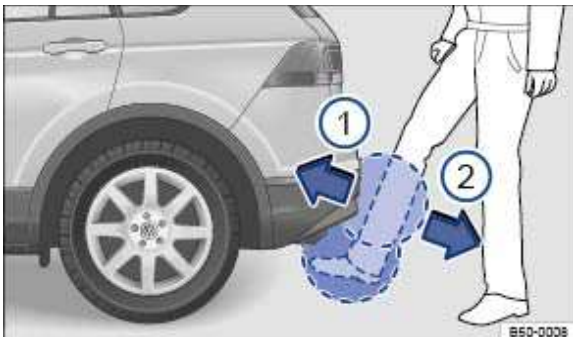
Fig. 84 Sensor-controlled luggage compartment opener (Easy Open).
