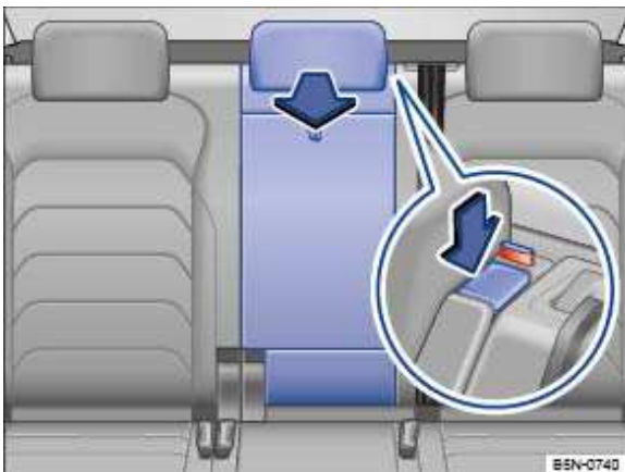
Fig. 222 In the rear seat backrest: opening the load-through hatch.
