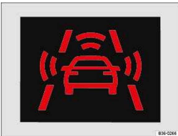
Fig. 163 On the instrument cluster display: advance warning display.
