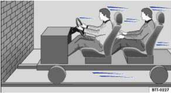
Fig. 4 Unbelted occupants in a vehicle heading for a brick wall.
