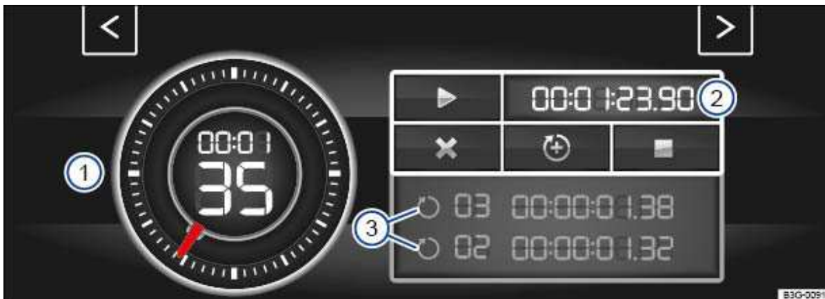
Fig. 62 On the infotainment system display: lap timer with stopwatch, function button and lap times.
