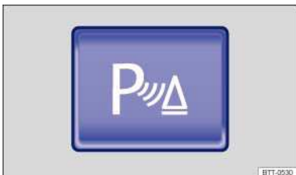
Fig. 175 In the centre console: button for switching the ParkPilot on and off (in some models).
