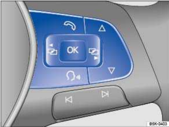
Fig. 59 Right-hand side of the multifunction steering wheel: buttons for using the menus and information displays in the instrument cluster display.
