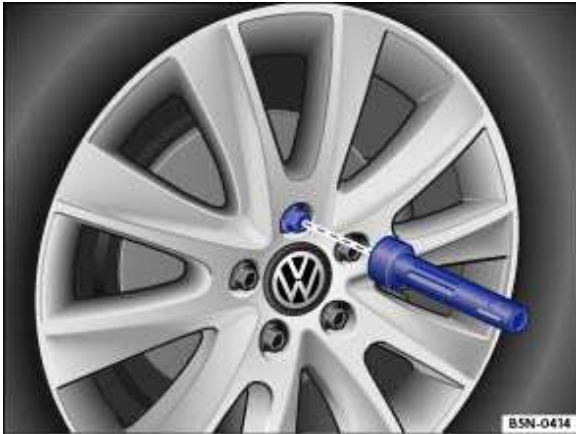
Fig. 278 Changing the wheel: removing the wheel bolts with the screwdriver handle.
