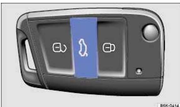
Fig. 81 In the vehicle key: button for unlocking the boot lid.
