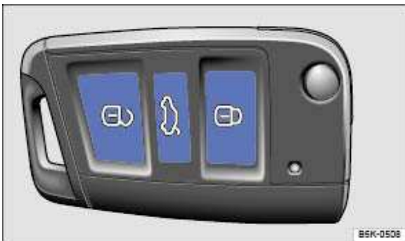
Fig. 68 Vehicle key: central locking system.
