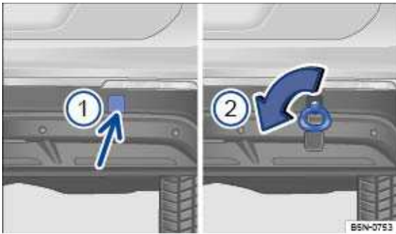
Fig. 252 On the right-hand side of the rear bumper: screwed-in towing eye.
