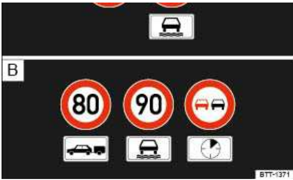
Fig. 53 On the instrument cluster display: examples of recognised speed limits or overtaking restrictions with accompanying additional signs.
