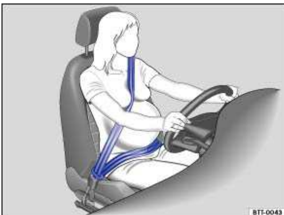
Fig. 12 Correct seat belt routing during pregnancy.
