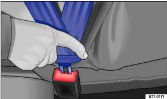
Fig. 9 Inserting the seat belt latch plate into the buckle.
