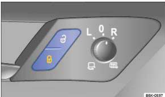
Fig. 69 In the driver door: central locking button.
