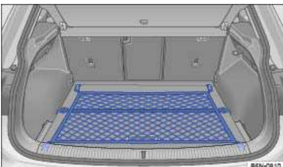
Fig. 220 In the luggage compartment: luggage net fastened to the luggage compartment floor.
