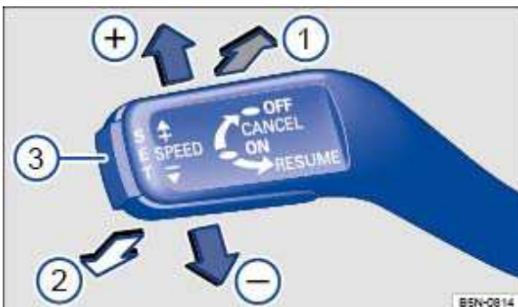
Fig. 152 On the left of the steering column: cruise control system lever.
