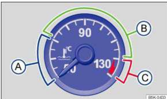
Fig. 55 In the instrument cluster: coolant temperature display (illustration).
