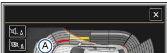
Fig. 178 ParkPilot screen displays: vehicle path displays without steering input.
