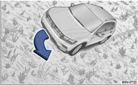
Fig. 148 Steering downhill along the maximum gradient.
