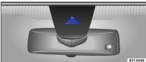
Fig. 168 Windscreen: lane keeping system camera window.
