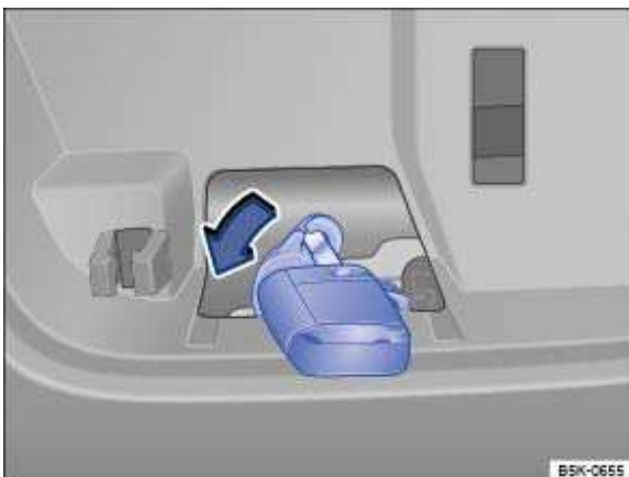
Fig. 86 In the luggage compartment: manual release for the boot lid.
