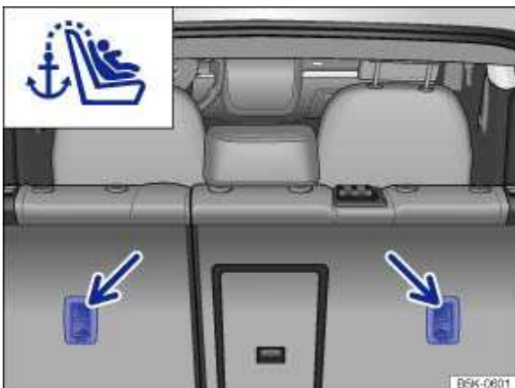
Fig. 28 Anchor rings for the top tether on the back of the rear bench seat.
