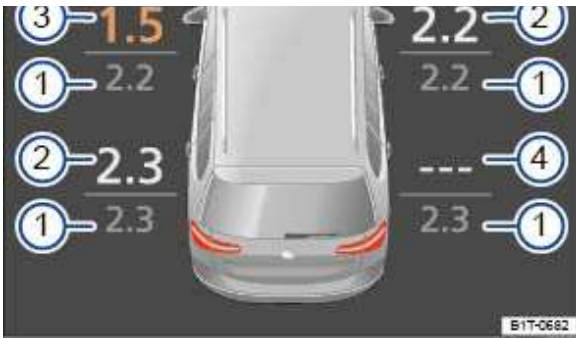
Fig. 264 Display in the instrument cluster: current tyre pressures.
