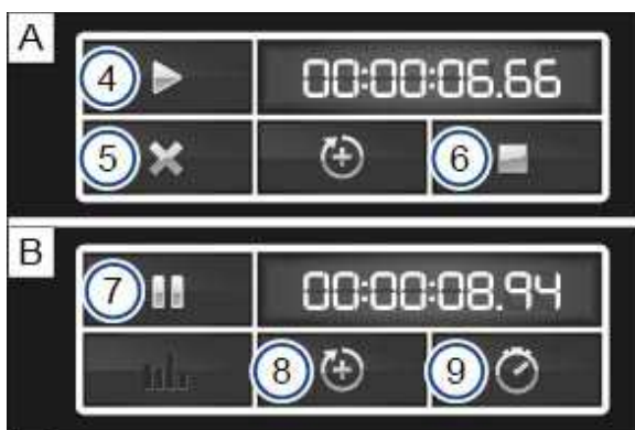
Fig. 62 On the infotainment system display: lap timer with stopwatch, function button and lap times.
