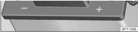
Fig. 263 A typical window on the top of the vehicle battery.
