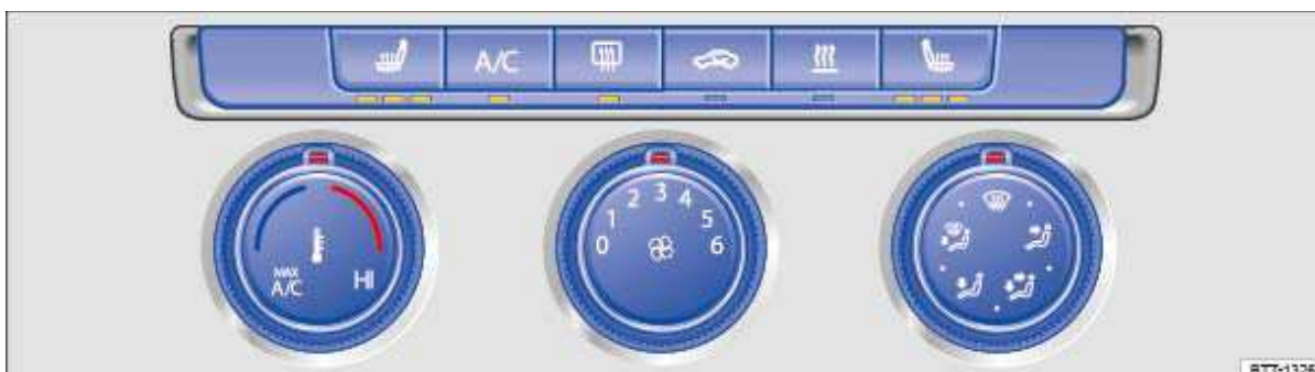
Fig. 121 In the upper part of the centre console: controls for the manual air conditioning system and/or heating and fresh air system.
