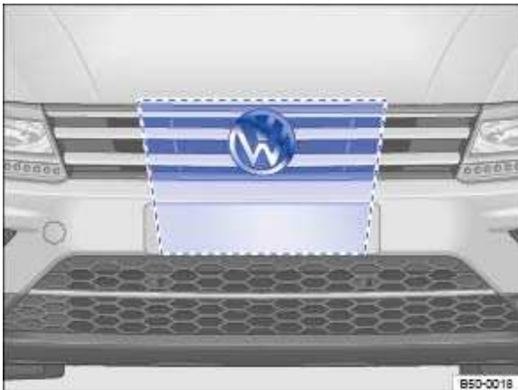
Fig. 164 In the radiator grille behind the Volkswagen badge: radar sensor and area around the radar sensor to be kept clear.
