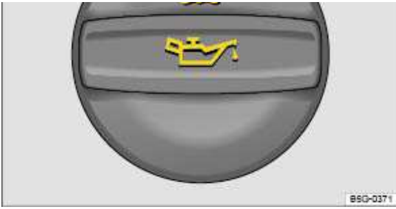
Fig. 258 In the engine compartment: engine oil filler cap (illustration).
