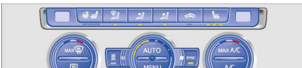
Fig. 121 In the upper part of the centre console: controls for the manual air conditioning system and/or heating and fresh air system.
