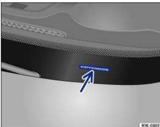
Fig. 281 In the windscreen: vehicle identification number.
