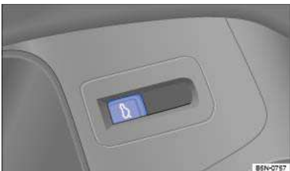
Fig. 70 In the driver door: release for the boot lid.
