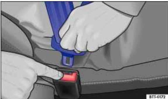
Fig. 10 Removing the latch plate from the buckle.
