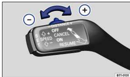
Fig. 273 Lever for Adaptive Cruise Control: Setting the distance (time intervals)
