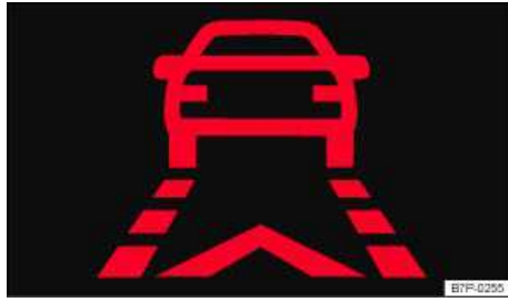
Fig. 276 In the instrument cluster display. Warning: Distance to vehicle ahead becoming too small.
