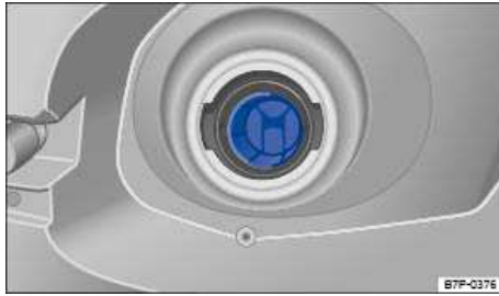
Fig. 307 With open fuel cap: Misfueling guard in the fuel filler neck.
