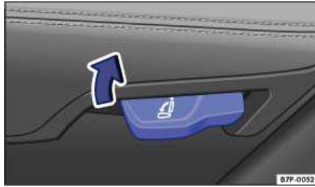
Fig. 99 Lower part of the rear seat bench: Lever to unlock the rear seat backrest by hand.
