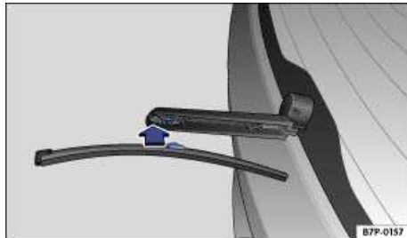
Fig. 322 Changing the rear window wiper blades.
