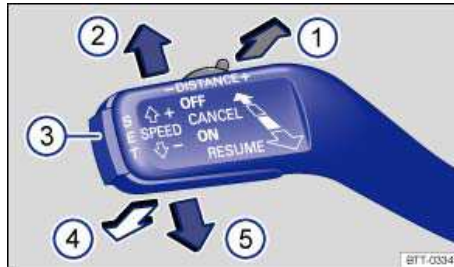
Fig. 272 On the steering wheel column: Lever for Adaptive Cruise Control.
