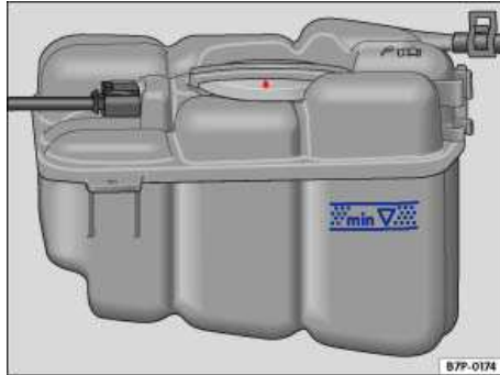
Fig. 319 Coolant expansion tank in the engine compartment.
