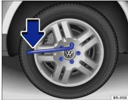
Fig. 337 Changing a wheel: Loosening wheel bolts.
