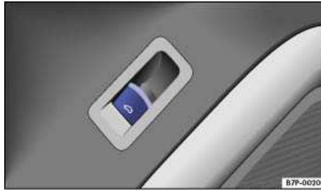
Fig. 30 In the driver door: Power button to unlock the rear hatch.
