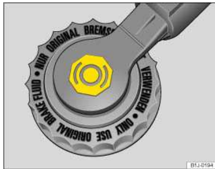
Fig. 254 In engine compartment: Brake fluid reservoir cap.
