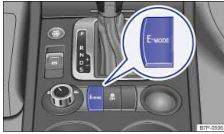
Fig. 257 In the lower center console: E-MODE button for extended electro-mode drive.
