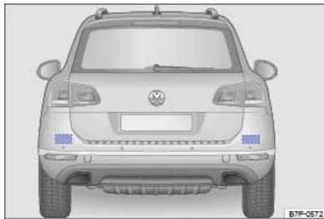
Fig. 281 Rear view of the vehicle: Areas of the Side Assist radar sensors.
