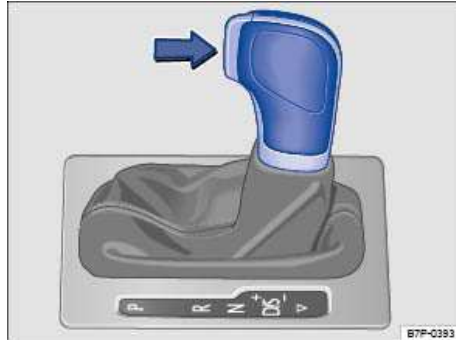
Fig. 249 Automatic transmission selector lever with shift lever release button (arrow).
