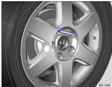
Fig. 342 Changing a wheel: Mounting pin in wheel bolt hole closest to the top.
