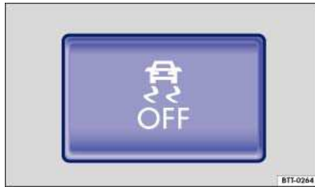
Fig. 253 In the front center console: Button to manually switch ASR on and off.
