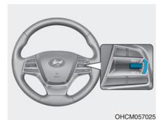
Push the toggle switch up (RES+) and hold it, while monitoring the SET speed on the instrument cluster.
