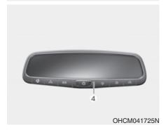
1. Press and hold the HomeLink button (1), (2) or (3), you would like to program. The HomeLink indicator light (4) will flash slowly in red (if not, perform the steps of "Erasing HomeLink Buttons" section, and start over).
