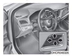
You can adjust the direction of air delivered from these vents using the vent control lever as shown.
