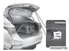
Your vehicle is equipped with an Emergency Trunk Safety Release lever located inside the trunk. When someone is inadvertently locked in the trunk, the trunk can be opened by moving the lever in the direction of the arrow and pushing the trunk open.
