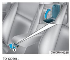
Grab and hold the latch (1) on the arm rest then lift the lid.
