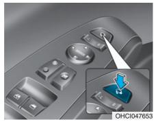
The side view mirrors can be folded or unfolder by pressing the switch.
