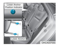
The lower anchor position indicator symbols are located on the left and right rear seat backs to identify the position of the lower anchors in your vehicle (see arrows in illustration).
