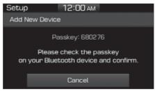
After confirming that the 6-digit passkey on the audio screen and the Bluetooth® Wireless Technology device are identical, select [OK] in your Bluetooth® Wireless Technology device.
