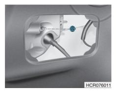
Loosen the lamp assembly retaining screws with a cross-tip screwdriver.
