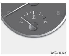
This gauge indicates the temperature of the engine coolant when the ignition switch is in the ON position.
