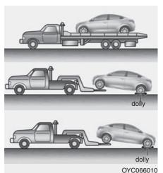
If emergency towing is necessary, have it done by an authorized HYUNDAI dealer or a commercial tow-truck service. Proper lifting and towing procedures are necessary to prevent damage to the vehicle. The use of wheel dollies or flatbed is recommended.
