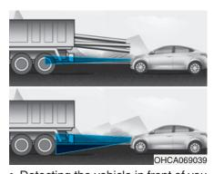
• Detecting the vehicle in front of you If the vehicle in front of you has cargo that extends rearward from the cab, or when the vehicle in front of you has higher ground clearance, additional special attention is required. FCA may not be able to detect the cargo extending from the vehicle. In these instances, you must maintain a safe braking distance from the rearmost object, and if necessary, depress the brake pedal to reduce your driving speed in order to maintain distance.
