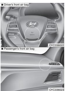
The purpose of the SRS is to provide the vehicle's driver and front passengers with additional protection than that offered by the seat belt system alone. The advanced SRS offers the ability to control the air bag inflation within two levels. A first stage level is provided for moderate-severity impacts.
