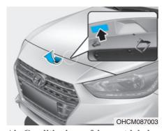
Air Conditioning refrigerant label You can find out which air conditioning refrigerant is applied to your vehicle on the label located inside of the hood.
