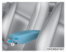
To move the armrest forward: Pull up the latch (1) then pull the armrest forward.
