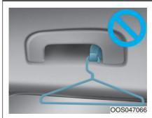
Do not hang other objects such as hangers or hard objects except clothes. Also, do not put heavy, sharp or breakable objects in the clothes pockets. In an accident or when the curtain air bag is inflated, it may cause vehicle damage or personal injury.
