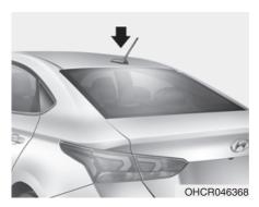
The roof antenna receives AM/FM signals.
