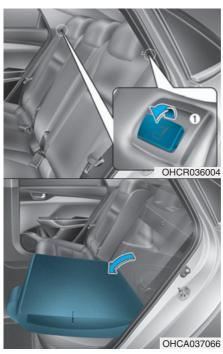
Pull up the seatback folding lever (1), then fold the seat toward the front of the vehicle.
