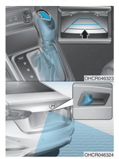
Rear View Monitor will activate when the engine is running and the shift lever is in the R (Reverse) position. This is a supplemental system that helps provide a view of the area behind the vehicle through the audio display while the vehicle is in the R (Reverse) position.
