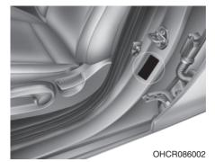
The vehicle certification label attached on the driver's side center pillar gives the Vehicle Identification Number (VIN).
