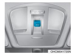
The sunroof can only be operated when the ignition switch is in the ON position.
