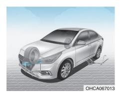
Block both the front and rear of the tire diagonally opposite of the tire you are changing.
