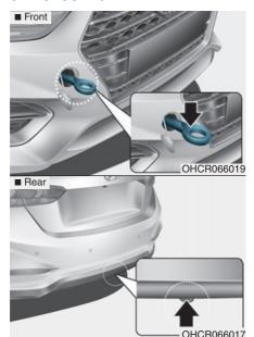
If towing is necessary, have it done by an authorized HYUNDAI dealer or a commercial tow truck service. If a towing service is not available in an emergency, your vehicle may be temporarily towed using a cable or chain secured to the emergency towing hook at the front (or rear) of the vehicle.
