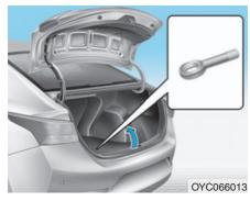
1. Open the trunk, and remove the towing hook from the tool case.
