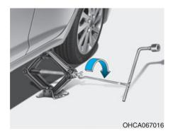
Insert the jack handle into the jack and turn it clockwise, raising the vehicle until the tire clears the ground. Make sure the vehicle is stable on the jack.
