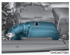
The air cleaner filter can be cleaned for inspection using compressed air. Do not attempt to wash or to rinse it, as water will damage the filter. If soiled, the air cleaner filter must be replaced.
