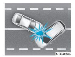
In an angled collision, the force of impact may direct the occupants in a direction where the air bags would not be able to provide any additional benefit, and thus the sensors may not deploy any air bags.
