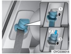
To adjust the height of the seat belt anchor, lower or raise the height adjuster into an appropriate position. To raise the height adjuster, pull it up
