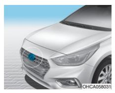
In order for FCA to operate properly, always make sure the sensor cover or sensor is clean and free of dirt, snow, and debris. Dirt, snow, or foreign substances on the sensor cover or sensor may adversely affect the sensing performance of the sensor.
