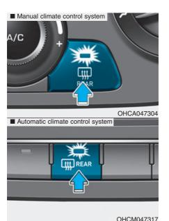
The defroster heats the window to remove frost, fog and thin ice from the interior and exterior of the rear window, while the engine is running.
