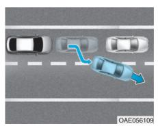
When driving in stop-and-go traffic, and a stopped vehicle in front of you merges out of the lane, FCA may not immediately detect the new vehicle that is now in front of you. In this case, you must maintain a safe braking distance, and if necessary, depress the brake pedal to reduce your driving speed in order to maintain a safe distance.
