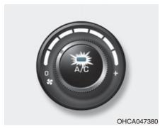
Push the A/C button to turn the system on (indicator light will illuminate) and off.
