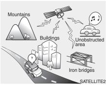
The signal can become weak in some areas that are not covered by the XM<sup>™</sup> repeater network.
