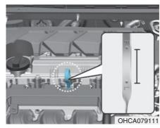
Pull the dipstick out again and check the level. The level should be between F and L.
