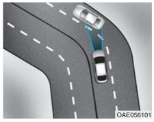
The front radar sensor recognition system may not detect the vehicle traveling in front on a curved road.
