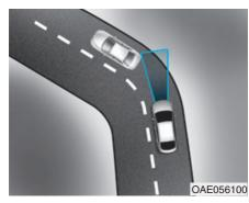
The front radar sensor recognition system may not detect the vehicle traveling in front on a curved road.
