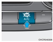
Push the A/C button to manually turn the system on (indicator light will illuminate) and off.
