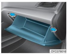
1. With the glove box open, lower the glove box by pushing both sides.
