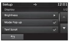
This feature is used to display the Pop-up Mode screen when entering radio and media modes.
