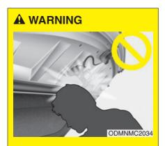
When you check the engine compartment, please make sure your head is not injured by the hood safety hook which is located inside of the hood.
