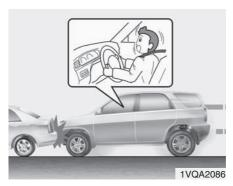
In certain low-speed collisions the air bags may not deploy. The air bags are designed not to deploy in such cases because they may not provide benefits beyond the protection of the seat belts in such collisions.
