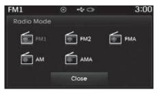
If [Pop-up Mode] is turned on within SETUP > [Display], then pressing the RADIO key will display the Radio Pop-up Mode screen.
