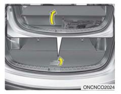
You can place a first aid kit, a reflector triangle, tools, etc. in the box for easy access.
