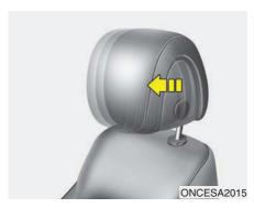
The headrest may be adjusted forward to 4 different positions by pulling the headrest forward to the desired detent. To adjust the headrest to it's furthest backwards position, pull the headrest to the desired detent while pushing the release button. Adjust the headrest so that it properly supports the head and neck.
