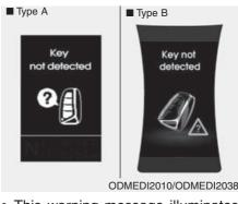
This warning message illuminates if the smart key is not detected when you press the Engine Start/Stop Button.
