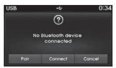
If Bluetooth® Wireless Technology devices are paired but none are currently connected, pressing the PHONE key or the key on the steering wheel displays the following screen. Press the [Pair] button to pair a new device or press the [Connect] to connect a previously paired.
