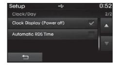
This feature is used to display a clock on the screen when the audio system is turned off.
