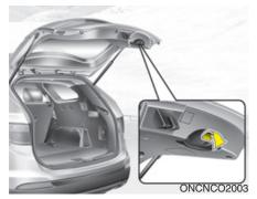
Lower and push down the tailgate firmly. Make sure that the tailgate is securely latched.
