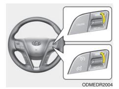
If any method other than the CAUISE button was used to cancel cruising speed and the system is still activated, the most recent set speed will automatically resume when you move the lever up (to RES+).
