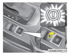
To apply the EPB (electric parking brake):
