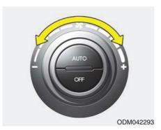
The fan speed control knob allows you to control the fan speed of the airflow in the vehicle.
