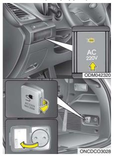
The AC inverter supplies 220V/200W electric power to operate electric accessories or equipments.
