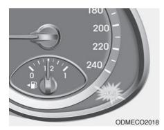
If the AFLS malfunction indicator comes on, the AFLS is not working properly. Drive to the nearest safe location and restart the engine. If the indicator continuously remains on, we recommend that you take your vehicle to an authorized HYUNDAI dealer and have the system checked.
