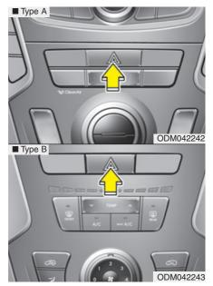
The hazard warning flasher should be used whenever you find it necessary to stop the car in a hazardous location. When you must make such an emergency stop, always pull off the road as far as possible. The hazard warning lights are turned on by pushing in the hazard switch. This causes all turn signal lights to blink. The hazard warning lights will operate even though the key is not in the ignition switch.
