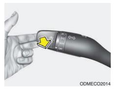
Pull the lever towards you. It will return to the normal position when released. The headlight switch does not need to be on to use this flashing feature.
