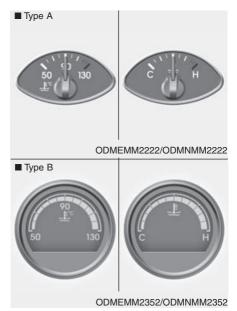
This gauge indicates the temperature of the engine coolant when the ignition switch or Engine Start/Stop button is ON.
