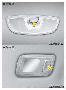
Press the button to turn the light on or off.
