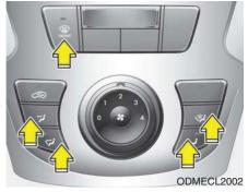
The mode buttons control the direction of the air flow through the ventilation system.
