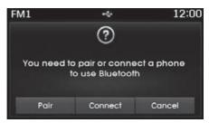
If Bluetooth® Wireless Technology devices are paired but none are currently connected, pressing the PHONE key or the key on the steering remote controller displays the following screen. Press the [Pair] button to pair a new device or press the [Connect] to connect a previously pair device.
