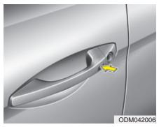
Carrying the smart key, you may lock and unlock the vehicle doors and tailgate.
