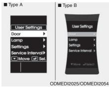
On this mode, you can change setting of the doors, lamps, and so on.
