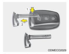
If the smart key does not operate normally, you can lock or unlock the doors by using the mechanical key.
