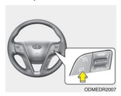
Press the speed limit (5) button on the steering wheel, to turn the system on.
