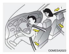
Your vehicle is equipped with driver's and front passenger's pre-tensioner seat belts (retractor pretensioner and EFD (Emergency Fastening Device)). The pre-tensioner seat belts can be activated, where the frontal collision is severe enough, together with the air bags.
