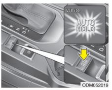
1.With the driver's door, engine hood and tailgate/trunk closed, fasten the driver's seat belt or depress the brake pedal and then press the Auto Hold button. The white AUTO HOLD indicator will come on and the system will be in the standby position.
