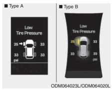
This warning message illuminates if the tire pressure is low with the Engine/Start button in ON position.
