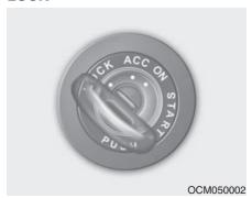
The steering wheel locks to protect against theft. The ignition key can be removed only in the LOCK position. When turning the ignition switch to the LOCK position, push the key inward at the ACC position and turn the key toward the LOCK position.
