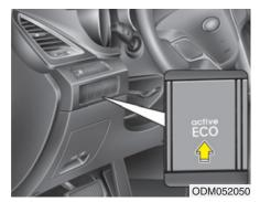
Active ECO helps improve fuel efficiency by controlling certain engine and transaxle system operating parameters. Fuel efficiency depends on the driver's driving habit and road condition.
