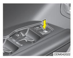
The driver can disable the power window switches on the rear passengers' doors by pressing the power window lock switch to the lock position (pressed).
