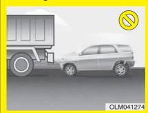
An accident may occur when parking behind a vehicle higher than yours. For example, bus, truck, etc.
