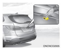
• Press the tailgate handle switch carrying the smart key with you.
