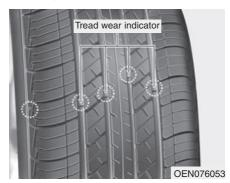
If the tire is worn evenly, a tread wear indicator will appear as a solid band across the tread. This shows there is less than 1.6 mm (1/16 in.) of tread left on the tire. Replace the tire when this happens.
