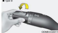
When the light switch is in the headlight position the head, tail, position, license and instrument panel lights are ON.
