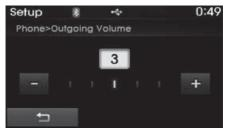
Use the \_\_\_, \_\_ buttons to adjust the outgoing volume level.
