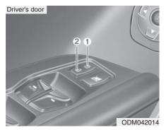
Operate by depressing the central door lock switch.
