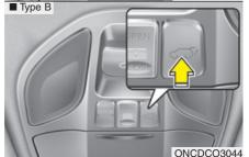
Press the power tailgate close button for approximately one second when the tailgate is opened.
