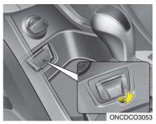
If your vehicle has an aux and/or USB (universal serial bus) port, you can use an aux port to connect audio devices and an USB port to plug in an USB and also in an iPod<sup>®</sup>.
