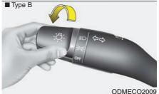
When the light switch is in the parking light position, the tail, position, license and instrument panel lights are ON.
