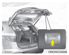
Press the power tailgate close button for approximately one second when the tailgate is opened.
