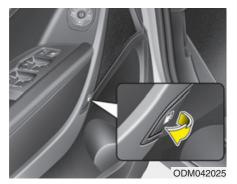
The fuel-filler lid must be opened from inside the vehicle by pulling up on the fuel-filler lid opener located on the driver's door.
