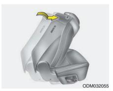
3. The 2nd row seatback will be folded and push the seat to the farthest forward position.
