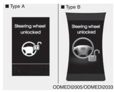
This warning message illuminates if the steering wheel does not lock when the Engine Start/Stop Button changes to the OFF position.
