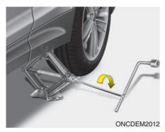
8. Insert the jack handle into the jack and turn it clockwise, raising the vehicle until the tire just clears the ground. This measurement is approximately 30 mm (1.2 in). Before removing the wheel lug nuts, make sure the vehicle is stable and that there is no chance for movement or slippage.
