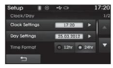
This feature is used to change the clock format between 12hr or 24hr.
