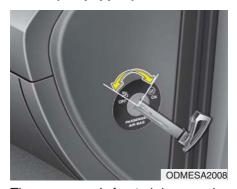
The passenger's front air bag can be deactivated by the passenger's front air bag ON/OFF switch if a child restraint is installed on the front passenger's seat or if the front passenger's seat is unoccupied by a person. To ensure the safety of your child, the passenger's front air bag must be deactivated when it should be necessary to install a rearward facing child seat on the front passenger seat in exceptional circumstances.
