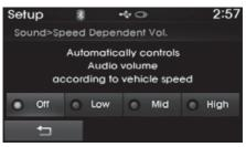
The volume level is controlled automatically according to the vehicle speed. SDVC can be set by selecting from Off/Low/Mid/High.
