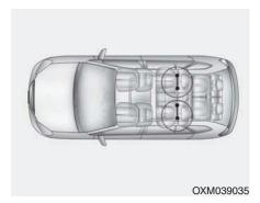
ISOFIX is a standardised method of fitting child seats that eliminates the need to use the standard adult seat belt to secure the seat in the vehicle. This enables a much more secure and positive location with the added benefit of easier and quicker installation.
