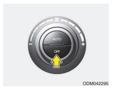
Press the blower OFF button to turn off the air climate control system. However, you can still operate the mode and air intake buttons as long as the ignition switch is in the ON position.
