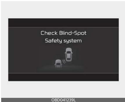
When Blind-Spot Collision-Avoidance Assist is not working properly, the 'Check Blind-Spot Safety system' warning message will appear (turns off after a certain time), and
