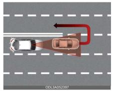
If the vehicle in front makes a sharp turn, such as to turn left or right or make a Uturn, etc., Leading Vehicle Departure Alert may not operate properly.
