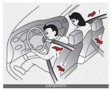
Your vehicle is equipped with driver's and front passenger's pre-tensioner seat belts (retractor pre-tensioner and EFD (Emergency Fastening Device). The pretensioner seat belts may be activated, when a frontal collision is severe enough, together with the air bags, depending on the crash severity, angle, speed and point of impact of the frontal collision.
