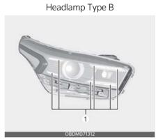
If the position lamp/daytime running lamp (LED) (1) does not operate, have the vehicle checked by an authorized Kia dealer.
