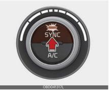
Press the "SYNC" button to adjust the driver and passenger side temperature equally. The passenger side temperature will be set to the same temperature as the driver side temperature.
