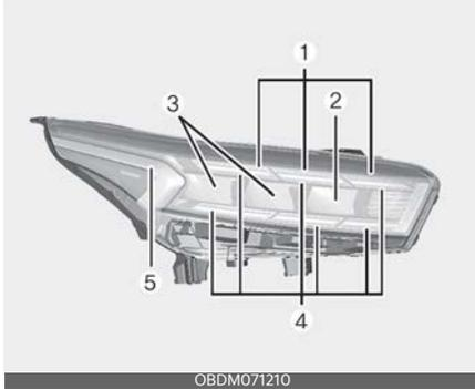
If the Front turn signal lamp (1), High beam lamp (2), Low beam lamp (3), Day time running lamp/Position lamp(4), side marker (5) does not operate, have the vehicle checked by an authorized Kia dealer.
