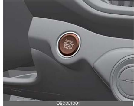
Whenever the front door is opened, the ENGINE START/STOP button will illuminate for your convenience. The light will go off after about 30 seconds when the door is closed. It will also go off immediately when the theft-alarm system is armed.
