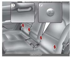
The LATCH anchors are located between the seatback and the seat cushion of the rear seat left and right outboard seating positions.
