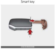
To reinstall the mechanical key, put the key into the hole and push it until a click sound is heard.
