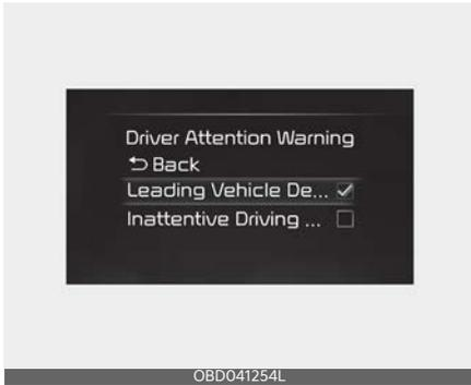
If 'Leading Vehicle Departure Alert' is selected, the function will inform the driver when a detected vehicle in front departs from a stop.
