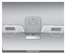
Air bag warning labels, some required by the U.S. National Highway Traffic Safety Administration (NHTSA), are attached to the sun visor to alert the driver and passengers of potential risks of the air bag system.
