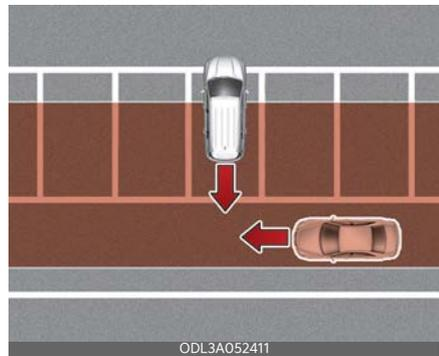
Rear Cross-Traffic Collision Warning may detect vehicles passing by behind you when parking backwards into a parking space. If this occurs, the function may unnecessarily warn the driver.
