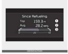
This display shows the accumulated trip distance (1), the average fuel efficiency
