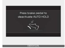
When you press the [AUTO HOLD] switch, if the driver's door, trunk, and engine hood are not closed, a warning will sound and a message will appear on the LCD display.
