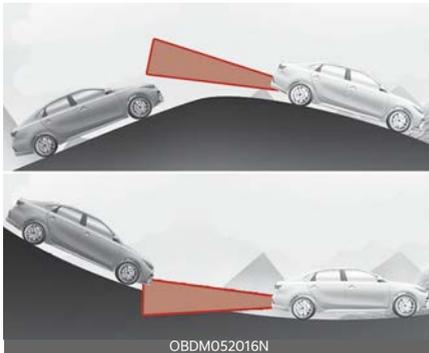
Blind-Spot Collision-Avoidance Assist may not operate properly when driving on a slope. The function may not detect the vehicle in the next lane or may incorrectly detect the ground or structure. Always pay attention to road and driving conditions while driving.
