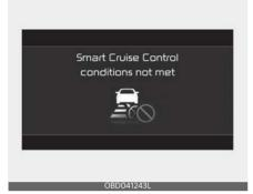
If the Driving Assist button, +, - or || switch is operated when Smart Cruise Control's operating conditions are not satisfied, the 'Smart Cruise Control conditions not met' will appear on the cluster, and an audible warning will sound.
