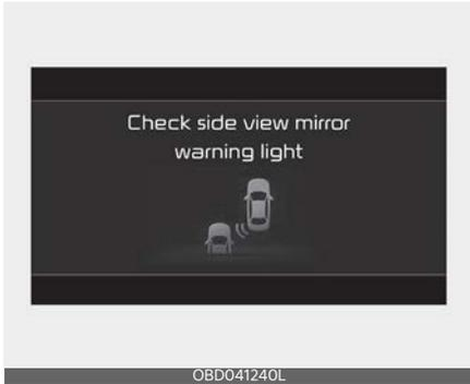
When the side view mirror warning light is not working properly, the 'Check side view mirror warning light' warning message will appear on the cluster. In this case, have your vehicle inspected by an authorized Kia dealer.
