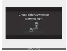
When the warning light on the side view mirror (outside mirror) is not working properly, the 'Check side view mirror warning light' warning message will appear (turns off after a certain time), and the  $\bigwedge$  warning light will illuminate on the cluster. In this case, have your vehicle inspected by an authorized Kia dealer.
