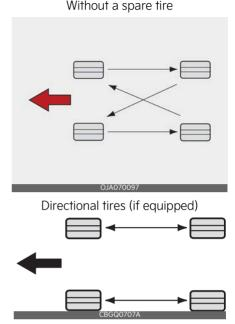
Rotate radial tires that have an asymmetric tread pattern only from front to rear and not from right to left.
