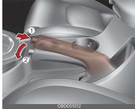
To release the parking brake, first apply the foot brake and pull up the parking brake lever slightly. Secondly depress the release button (1) and lower the parking brake lever (2) while holding the button.
