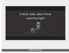
When the outside rear view mirror warning light is not working properly, the 'Check side view mirror warning light' warning message will appear on the cluster for several seconds, and the master (\u03c6) warning light will appear on
