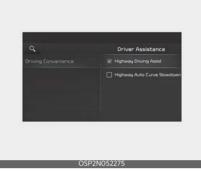
With the ignition switch or ENGINE START/STOP button in the ON position, select 'Driver Assistance  $\rightarrow$  Driving Convenience' from the Setup menu to set whether to use each function.
