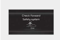
When Forward Collision-Avoidance Assist is not working properly, the 'Check Forward Safety system' warning message will appear (turns off after a
