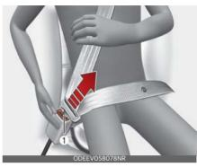
• Press the release button (1) in the locking buckle.
