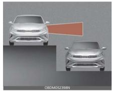
Blind-Spot Collision Warning may not operate properly when driving where the heights of the lanes are different. The function may not detect the vehicle on a road with different lane heights (underpass joining section, grade separated intersections, etc.). Always pay attention to road and driving conditions while driving.
