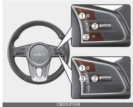
The LCD display modes can be changed by using the control buttons on the steering wheel.
