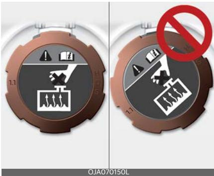
2. Make sure that the tiny protrusions inside the coolant cap are securely interlocked.
