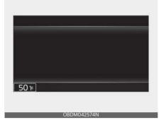
This gauge indicates the current outside air temperatures by 1°F (1°C).
