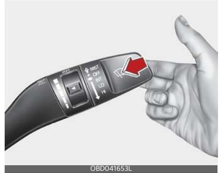
1. Move the wiper speed control switch to OFF position.
