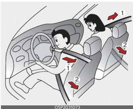
Your vehicle is equipped with driver's and front passenger's pre-tensioner seat belts (retractor pre-tensioner and EFD (Emergency Fastening Device)). The pre-tensioner seat belts may be activated,
