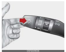
It will return to the normal (low beam) position when released. The head-
