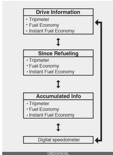
To change the trip mode, scroll the toggle the switch (∧ / ∨) on the steering wheel.
