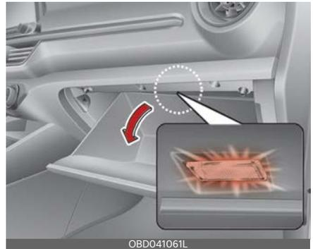
The glove box lamp comes on when the glove box is opened.
