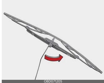
2. Compress the clip (1) and slide the blade assembly (2) downward.
