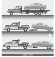
If any of the loaded wheels or suspension components are damaged or the vehicle is being towed with the front wheels on the ground, use a towing dolly under the front wheels.
