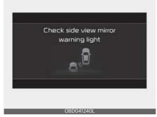
When the side view mirror warning light is not working properly, the 'Check side view mirror warning light' warning message will appear on the cluster. In this case, have your vehicle inspected by an authorized Kia dealer.
