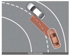
Blind-Spot Collision-Avoidance Assist may not operate properly when driving on the curved road. The function may recognize the vehicle in the same lane. Always pay attention to road and driving conditions while driving.
