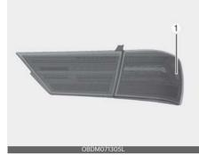
If the side marker (LED) (1) does not operate, have the vehicle checked by an authorized Kia dealer. The LED lamp cannot be replaced as a single component because it is an integrated unit. The LED lamp has to be replaced with the unit. A skilled technician should check or repair the side marker (LED), for it may damage related parts of the vehicle.
