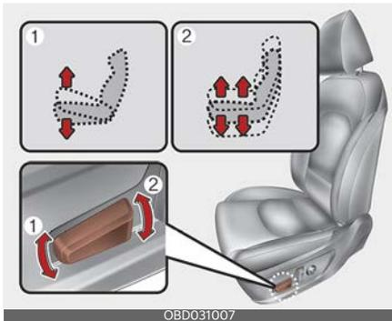
1. Pull the front portion (1) of the control switch up to raise or press down to lower the front part of the seat cushion.
