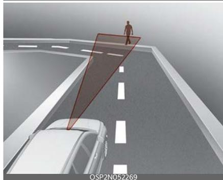
Forward Collision-Avoidance Assist may detect a vehicle or pedestrian in the next lane or outside the lane when driving on a curved road.
