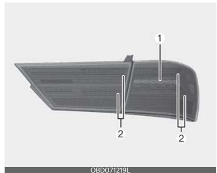
If the stop (1) and tail (2) lamp (LED), does not operate, have the vehicle checked by an authorized Kia dealer. The LED lamps cannot be replaced as a single unit because it is an integrated unit. The LED lamps has to be replaced with the unit.
