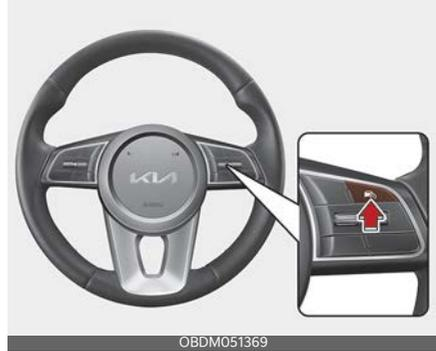
Press the Driving Assist button to turn Manual Speed Limit Assist off. The Speed Limit indicator will go off. Always press the Driving Assist button to turn Manual Speed Limit Assist off when not in use.
