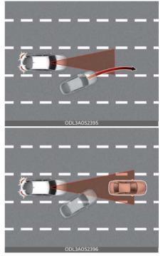
If a vehicle cuts in front of your vehicle, Leading Vehicle Departure Alert may not operate properly.
