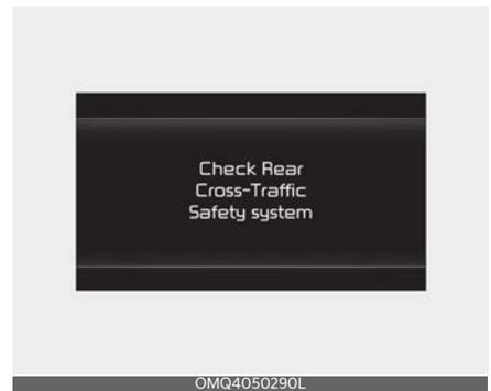
When Rear Cross-Traffic Collision Warning is not working properly, the 'Check Rear Cross-Traffic Safety system' warning message will appear on the cluster,
