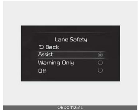
With the ignition switch or ENGINE START/STOP button in the ON position, select 'Driver Assistance → Lane Safety' from the 'User Settings (LCD display) or Setup → Vehicle (Infotainment System screen)' menu to set whether to use each function.
