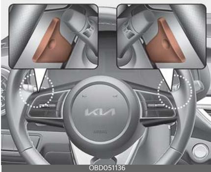
The paddle shifter is available when the shifter lever is in the D (Drive) position or the manual mode.
