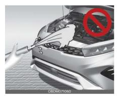
• Never allow water or other liquids to come in contact with electrical/electronic components inside the vehicle as this may damage them.
