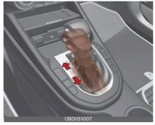
Whether the vehicle is stationary or in motion, manual mode is selected by pushing the shift lever from the D (Drive) position into the manual gate. To return to D (Drive) range operation, push the shift lever back into the main gate. Manual mode manages the driving dynamics by automatically adjusting the steering effort, and the engine and transmission control logic for enhanced driver performance.
