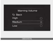
With the ignition switch or the ENGINE START/STOP button in the ON position, select 'Driver Assistance → Warning Volume' from the Settings menu to change the Warning Volume to 'High', 'Medium' or 'Low' for Reverse Parking Distance Warning.
