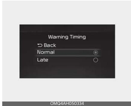
With the ignition switch or ENGINE START/STOP button in the ON position, select 'Driver Assistance → Warning Timing' from the 'User Settings (LCD display) or Setup → Vehicle (Infotainment System screen)' menu to change the initial warning activation time for Blind-Spot Collision-Avoidance Assist.
