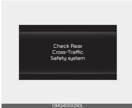
When Rear Cross-Traffic Collision-Avoidance Assist is not working properly, the 'Check Rear Cross-Traffic Safety system' warning message will appear (turns off after a certain time), and the
