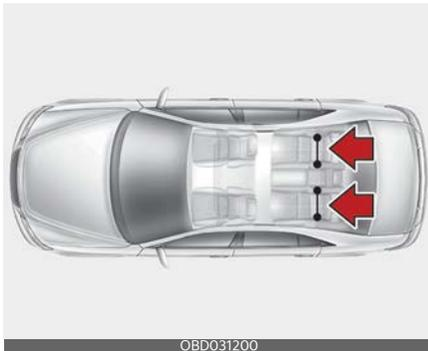
LATCH anchors have been provided in the left and right outboard rear seating positions. Their locations are shown in the illustration. There are no LATCH anchors provided for the center rear seating position.
