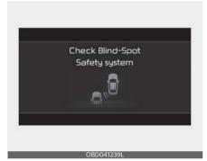
When Blind-Spot Collision-Avoidance Assist is not working properly, the 'Check Blind-Spot Safety system' warning message will appear (turns off after a certain time), and  $\bigwedge$  warning light will illuminate on the cluster. In this case, have your vehicle inspected by an authorized Kia dealer.
