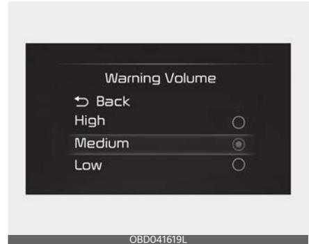
With the ignition switch or ENGINE START/STOP button in the ON position, select 'Driver Assistance → Warning Volume' from the 'User Settings (LCD display) or Setup → Vehicle (Infotainment System screen)' menu to change the Warning Volume to 'High', 'Medium' or 'Low' for Forward Collision-Avoidance Assist.
