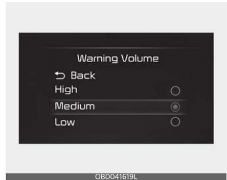
With the ignition switch or ENGINE START/STOP button in the ON position, and select 'User Settings (LCD display) or Settings → Vehicle (Infotainment System screen) → Driver Assistance → Warning Volume' to change the Warning Volume to 'High', 'Medium' or 'Low' for Safe Exit Warning.
