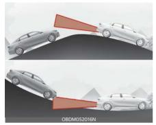
Blind-Spot Collision Warning may not operate properly when driving on a sloped road. The function may not detect the vehicle in the next lane or may incorrectly detect the ground or structure.
