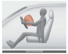
A fully inflated air bag, in combination with a properly worn seat belt, slows the driver's or the passenger's forward motion, reducing the risk of head and chest injury. Driver's front air bag (3)
