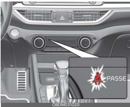
As a reminder to the front passenger, the front passenger's seat belt warning lights will illuminate for approximately 6 seconds each time you turn the ignition switch or the ENGINE START/STOP button in ON regardless of belt fastening. If the front passenger continue not to fasten the seat belt and drives below 12 mph (20km/h), the warning light will stay illuminated.
