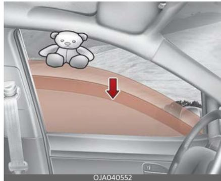
If the upward movement of the window is blocked by an object or part of the body, the window will detect the resistance and will stop upward movement. The window will then lower approximately 11.8 inches (30 cm) to allow the object to be cleared.
