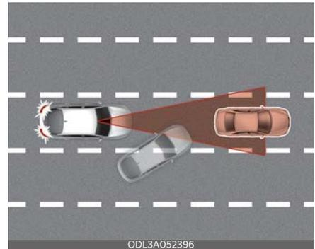
If a vehicle cuts in front of your vehicle, Leading Vehicle Departure Alert may not operate properly.
