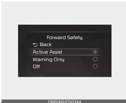
With the ignition switch or ENGINE START/STOP button in the ON position, select 'Driver Assistance → Forward Safety' from the 'User Settings (LCD display) or Setup → Vehicle (Infotainment
