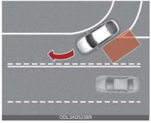
Blind-Spot Collision Warning may not operate properly when driving where the road merges or divides. The function may not detect the vehicle in the next lane.
