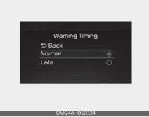
With the ignition switch or ENGINE START/STOP button in the ON position, select 'Driver Assistance → Warning Timing' from the 'User Settings (LCD display) or Setup → Vehicle (Infotainment System screen)' menu to change the initial warning activation time for Blind-Spot Collision-Avoidance Assist.
