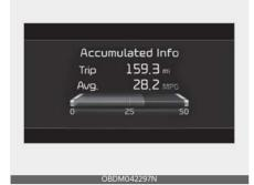
The trip computer mode displays information related to vehicle driving parameters including Accumulated info, Driving information, and so on.
