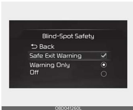
With the ignition switch or the ENGINE START/STOP button in the ON position, and select 'User Settings (LCD display) or Settings → Vehicle (Infotainment System screen) → Driver Assistance → Blind-Spot Safety → Safe Exit Warning' to turn on Safe Exit Warning and deselect to turn off the function.
