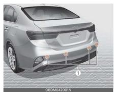
[1] : Rear ultrasonic sensors Refer to the picture above for the detailed location of the detecting sensors.
