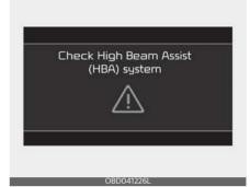
When High Beam Assist is not working properly, the warning message will come on for a few seconds. After the message disappears, the master warning light
