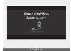
When Safe Exit Warning is not working properly, the 'Check Blind-Spot Safety system' warning message will appear on the cluster for several seconds, and the master ( ) warning light will illuminate on the cluster. In this case, have the vehicle inspected by an authorized Kia dealer.
