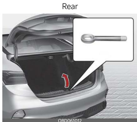
2. Remove the hole cover pressing the lower (front) part of the cover on the bumper.
