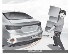
If you are positioned in the detecting area (20 ~ 40 inches (50 ~ 100 cm) behind the vehicle) carrying a smart key, the hazard warning lights will blink and chime will sound to alert you the smart key has been detected and the trunk will open.
