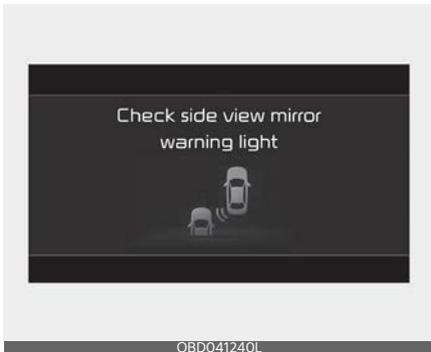
When the warning light on the side view mirror is not working properly, the 'Check side view mirror warning light' warning message will appear (turns off after a certain time), and
