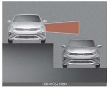
Blind-Spot Collision-Avoidance assist may not operate properly when driving where the heights of the lanes are different. The function may not detect the vehicle on a road with different lane heights (underpass joining section, grade separated intersections, etc.).
