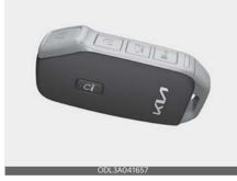
With a smart key, you can lock or unlock a door and even start the engine without inserting the key.
