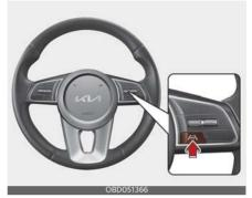
With the ignition switch or ENGINE START/STOP button in the ON position, press the Lane Driving Assist button located on the steering wheel to turn on Lane Following Assist. The white or green () indicator light will illuminate on the cluster.
