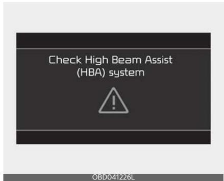
When High Beam Assist is not working properly, the warning message will come on for a few seconds. After the message disappears, the master warning light (⚠) will illuminate.
