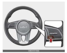
With the ignition switch or ENGINE START/STOP button in the ON position, press and hold the Lane Driving Assist button (
