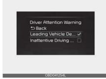
If 'Leading Vehicle Departure Alert' is selected, the function will inform the driver when a detected vehicle in front departs from a stop.
