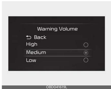
With the ignition switch or ENGINE START/STOP button in the ON position, select 'Driver Assistance → Warning Volume' from the 'User Settings (LCD display) or Setup → Vehicle (Infotainment System screen)' menu to change the Warning Volume to 'High', 'Medium' or 'Low' for Lane Keeping Assist.
