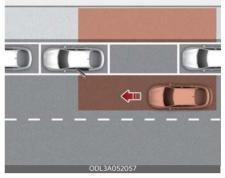
After the vehicle stops, when an approaching vehicle from the rear area is detected after a passenger opens the door, Safe Exit Warning will warn the driver with a warning message and an audible warning to help prevent a collision.
