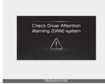
When Driver Attention Warning is not working properly, the 'Check Driver Attention Warning (DAW) system' warning message will appear on the cluster (turns off after a certain time) and  $\bigwedge$ warning light will illuminate. In this case,
