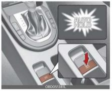
Before the Auto Hold will engage, the driver's door, trunk, and engine hood must be closed.
