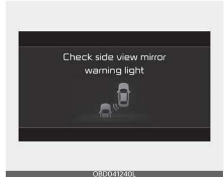
When the side view mirror warning light is not working properly, the 'Check side view mirror warning light' warning message will appear on the cluster. In this case, have your vehicle inspected by an authorized Kia dealer.
