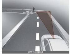
Forward Collision-Avoidance Assist may not detect other vehicle, pedestrian in front of you when driving on curved roads adversely affecting the performance of the sensors. This may result in no warning or no braking assist when necessary.
