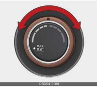
To change the air temperature in the passenger compartment, turn the knob to the right for warm and hot air or to the left for cooler air.
