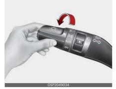
When the light switch is in the position lamp position, the front position lamp and, tail, license light will turn ON.
