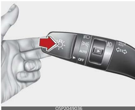
It will return to the normal (low beam) position when released. The head-
