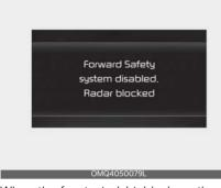
When the front windshield where the front view camera is located, front radar cover or sensor is covered with foreign material such as snow or rain, it can reduce the detecting performance and temporarily limit or disable Forward Collision-Avoidance Assist. If this occurs the 'Forward Safety system disabled. Radar blocked' warning message will appear (turns off after a certain time), and the
