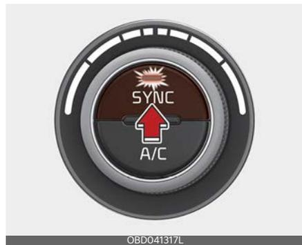
1. Press the "SYNC" button to adjust the driver and passenger side temperature equally.
