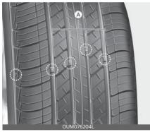
This shows there is less than 1/16 inch (1.6 mm) of tread left on the tire. Replace the tire when this happens.
