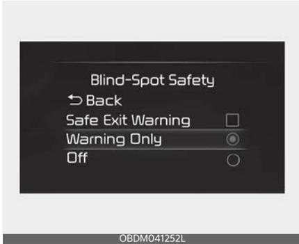
With the ignition switch or ENGINE START/STOP button in the ON position, select or deselect 'User Settings (LCD display) or Setup → Vehicle (Infotainment System screen) → Driver Assistance → Blind-Spot Safety' to set whether to use each function.
