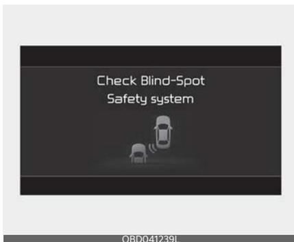
When Blind-Spot Collision Warning is not working properly, the 'Check Blind-Spot Safety system' warning message will
