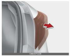
5. Remove the socket from the assembly by turning the socket counterclockwise until the tabs on the socket align with the slots on the assembly.
