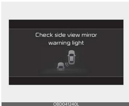
When the warning light on the side view mirror (outside mirror) is not working properly, the 'Check side view mirror warning light' warning message will
