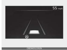
If the vehicle ahead or both lane markings are detected and your vehicle speed is below 110 mph (180 km/h), the green () indicator light will illuminate on the cluster, and the function will help center the vehicle in the lane by controlling the steering wheel.
