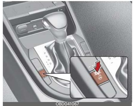
To turn the heated steering wheel off, press the button once again. The indicator on the button will turn off.
