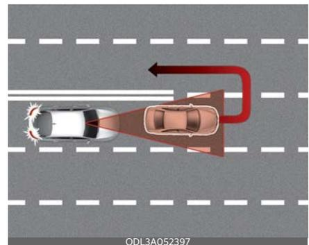
If the vehicle in front makes a sharp turn, such as to turn left or right or make a U-turn, etc., Leading Vehicle Departure Alert may not operate properly.
