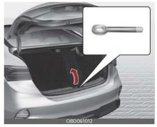
2. Remove the hole cover pressing the lower (front) part of the cover on the bumper.
