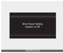
When the engine is restarted with the function off, the 'Blind-Spot Safety System is Off' message will appear on the cluster.
