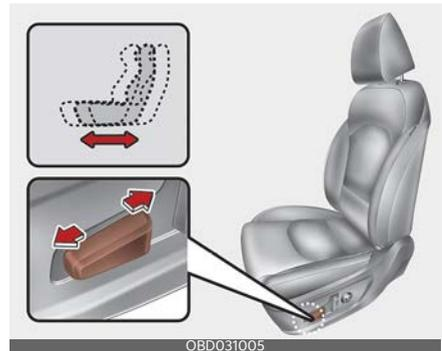
1. Push the control switch forward or backward to move the seat to the desired position.
