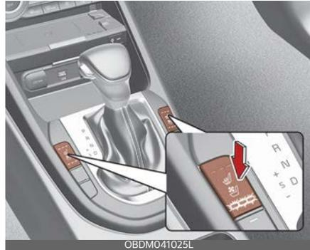
The temperature setting of the seat changes according to the button position.
