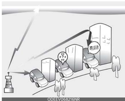
AM and FM radio signals are broadcast from transmitter towers located around your city. They are intercepted by the
