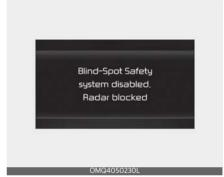
When the rear bumper around the rear corner radar or sensor is covered with foreign material, such as snow or rain, or installing a trailer or carrier, it can reduce the detecting performance and temporarily limit or disable Blind-Spot Collision-Avoidance Assist.
