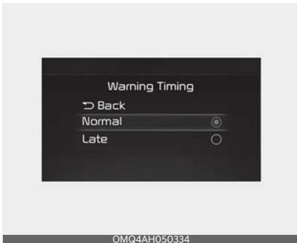
With the ignition switch or ENGINE START/STOP button in the ON position, select 'Driver Assistance → Warning Timing' from the 'User Settings (LCD display) or Setup → Vehicle (Infotainment System screen)' menu to change the ini-
