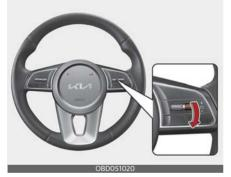
Push the + switch up or - switch down and hold it. The speed will increase or decrease to the nearest multiple of five (multiple of ten in km/h) at first, and then increase or decrease by 5 mph (10 km/h).
