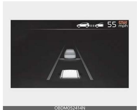
If temporary deceleration is required in the standby state and Navigation-based Smart Cruise Control is operating, the green (AUTO) symbol will illuminate on the cluster.
