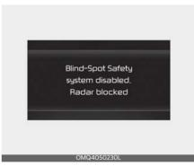
When the rear bumper around the rear corner radar or sensor is covered with foreign material, such as snow or rain, or installing a trailer or carrier, it can reduce the detecting performance and temporarily limit or disable Blind-Spot Collision Warning.
