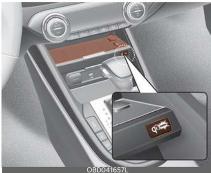
Firmly close all doors, and the ignition switch or ENGINE START/STOP button is ON. To start wireless charging, place the smart phone equipped with wireless
