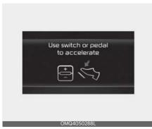
In traffic, your vehicle will stop if the vehicle ahead of you stops. Also, if the vehicle ahead of you starts moving, your vehicle will start as well. In addition, after the vehicle has stopped and a certain time has passed, the 'Use switch or pedal to accelerate' message will appear on the cluster. Depress the accelerator pedal or operate the + switch, - switch or ||  $\bigcirc$  switch to start driving.
