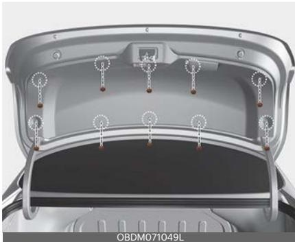
2. Loosen the retaining screw of the trunk lid cover and then remove the cover.
