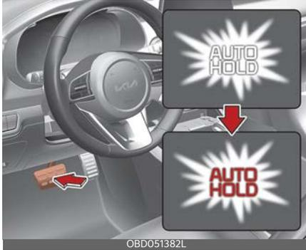
When coming to a complete stop by depressing the brake pedal, the AUTO HOLD indicator changes from white to green indicating the AUTO HOLD is engaged. The vehicle will remain at a standstill even if you release the brake pedal.
