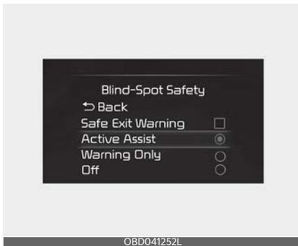
With the ignition switch or ENGINE START/STOP button in the ON position, select 'Driver Assistance → Blind-Spot Safety' from the 'User Settings (LCD display) or Setup → Vehicle (Infotainment System screen)' menu to set whether to use each function.
