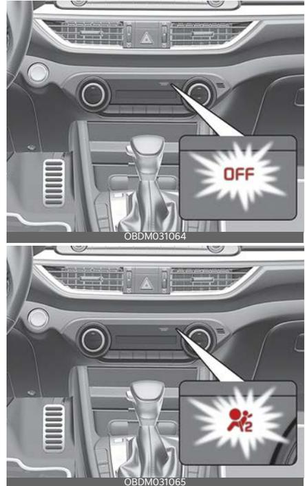
Your vehicle is equipped with an occupant detection system in the front passenger's seat.
