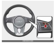
Press the Driving Assist button to turn Manual Speed Limit Assist off. The Speed Limit indicator will go off. Always press the Driving Assist button to turn Manual Speed Limit Assist off when not in use.
