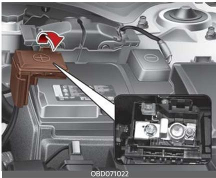
3. Replace the fuse with a new one of the same rating.
