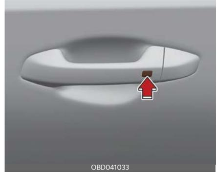
Pressing the button of the front driver side door handles with all doors (and trunk) closed and any door unlocked, locks all the doors (and trunk). If all doors (and trunk) and engine hood are closed, the hazard warning lights will blink once and the chime will sound once to indicate the vehicle is locked.
