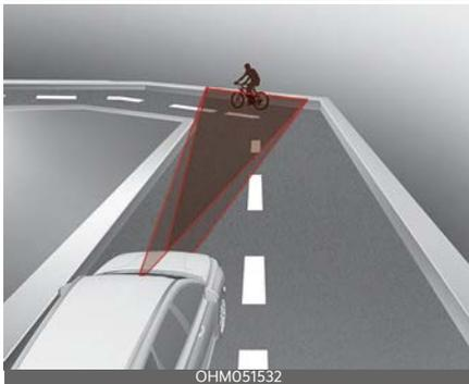
Forward Collision-Avoidance Assist may detect a vehicle or pedestrian in the next lane or outside the lane when
