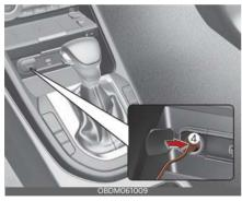
10.With the ignition switch or ENGINE START/STOP button position on: switch on the compressor and let it run for approximately 5~7 minutes to fill the sealant up to proper pressure. (Refer to "Tires and wheels" on page 7-35.) Be careful not to overinflate the tire and stay away from the tire when filling it. When the tire and wheel are damaged, do not use Tire Mobility Kit for your safety.
