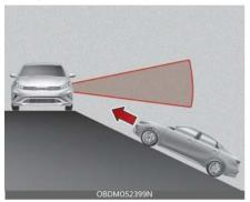
Rear Cross-Traffic Collision Warning may be limited when the vehicle is on a uphill or downhill slope, or near it, and may not detect the vehicle approaching from the left or right. If this occurs, the function may not warn the driver when necessary.
