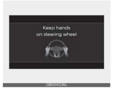
The hands-off warning appears when the function detects that the driver's hands are not on the steering wheel while Highway Driving Assist is in work.
