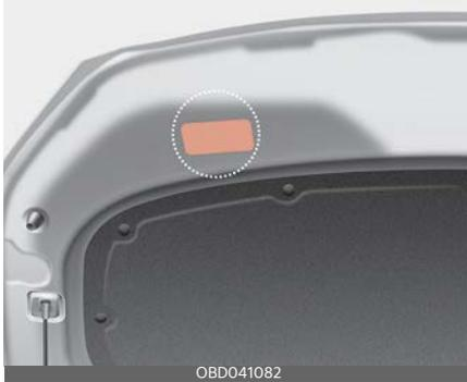
The refrigerant label is located on the underside of the hood.
