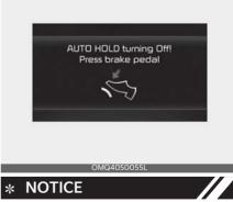
When this message is displayed, the Auto Hold and EPB may not operate. For your safety, depress the brake pedal.
