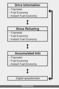
To change the trip mode, scroll the toggle the switch (///) on the steering wheel.
