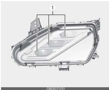
If the front fog lamp (LED) (1), does not operate, have the vehicle checked by an authorized Kia dealer. The LED lamps cannot be replaced as a single unit because it is an integrated unit. The LED lamps has to be replaced with the unit. A skilled technician should check or repair the front fog lamp (LED), for it may damage related parts of the vehicle.
