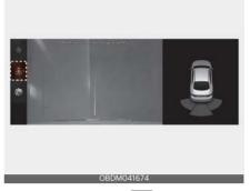
When you touch the ( ) icon, the top view is displayed on the screen and shows the distance from the vehicle in the back of your vehicle while parking.
