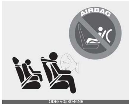
Never place a rear-facing child restraint in the front passenger's seat. If the air bag deploys, it would impact the rear-facing child restraint, causing serious or fatal injury.
