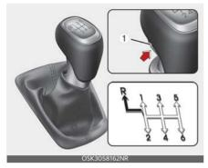
$\Box$  The shift lever can be moved without pushing the button (1).
