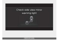
When the warning light on the side view mirror is not working properly, the 'Check side view mirror warning light' warning message will appear (turns off after a certain time), and  $\bigwedge$  warning light will illuminate on the cluster. In this case, have your vehicle inspected by an authorized Kia dealer.
