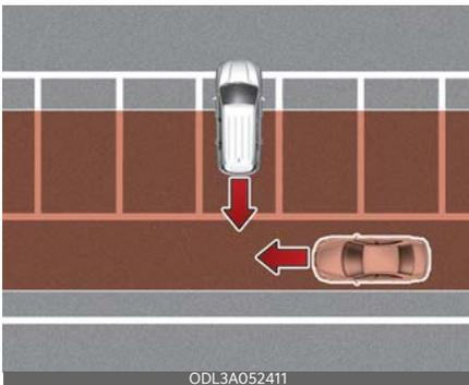
Rear Cross-Traffic Collision-Avoidance Assist may detect vehicles passing by behind you when parking backwards
