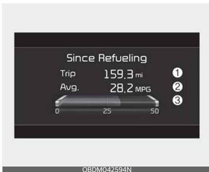
This display shows the accumulated trip distance (1), the average fuel efficiency
