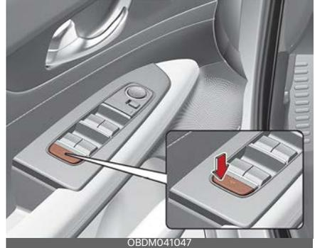
When the power window lock button is pressed:
