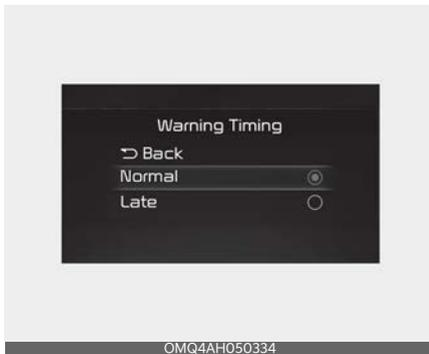
With the ignition switch or ENGINE START/STOP button in the ON position, select 'Driver Assistance → Warning Timing' from the 'User Settings (LCD display) or Setup → Vehicle (Infotainment System screen)' to change the initial warning activation time for Blind-Spot Collision Warning.
