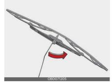
2. Compress the clip (1) and slide the blade assembly (2) downward.
