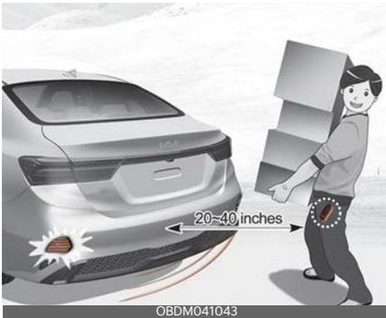
If you are positioned in the detecting area (20 ~ 40 inches (50 ~ 100 cm) behind the vehicle) carrying a smart key, the hazard warning lights will blink and chime will sound to alert you the smart key has been detected and the trunk will open.
