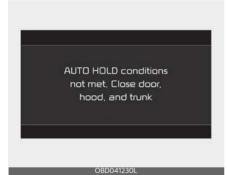
At this moment, press the [AUTO HOLD] button after closing the driver's door, engine hood and trunk.
