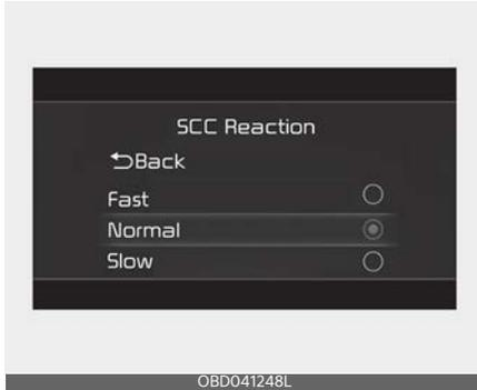
The sensitivity of vehicle speed when following the front vehicle to maintain the set distance can be adjusted. With the ignition switch or ENGINE START/STOP button in the ON position, select 'Driver Assistance → SCC Reaction' from the 'User Settings (LCD display) or Setup → Vehicle (Infotainment System screen)' menu to set one of the three stages you prefer.
