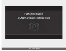
If the driver turns the engine off by mistake while Auto Hold (if equipped) is operating, EPB will be automatically applied. But if the driver turns the engine off and pushes the EPB switch for 1 second, the EPB does not apply.
