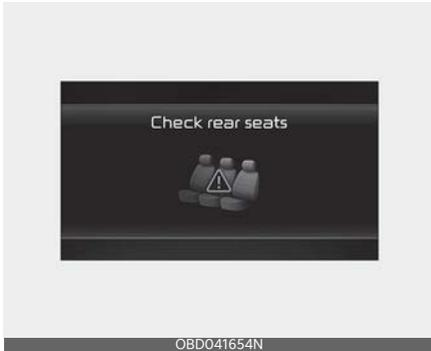
You can activate or deactivate the Rear Occupant Alert by selecting 'User Settings (LCD display) or Settings → Vehicle (Infotainment System screen) → Convenience → Rear Occupant Alert'.
