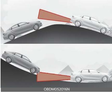
Blind-Spot Collision Warning may not operate properly when driving on a sloped road. The function may not detect the vehicle in the next lane or may incorrectly detect the ground or structure.
