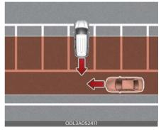
Rear Cross-Traffic Collision Warning may detect vehicles passing by behind you when parking backwards into a parking space. If this occurs, the function may unnecessarily warn the driver. Always check your surroundings while backing up.
