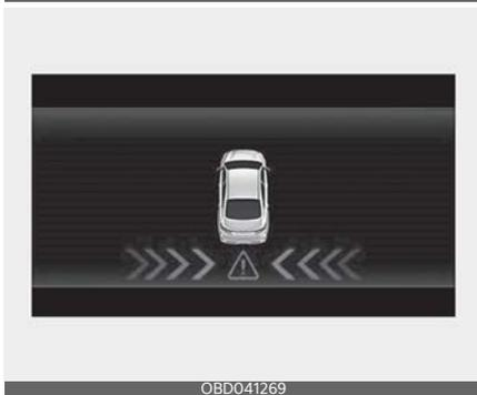
To warn the driver of an approaching vehicle from the rear left/right side of your vehicle, the side view mirror will blink and a warning will appear on the cluster. At the same time, an audible warning will sound. If Rear View Monitor is operating, a warning will also appear on the infotainment screen.
