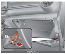
3. Remove the climate control air filter cover while pressing the lock on the left side of the cover.
