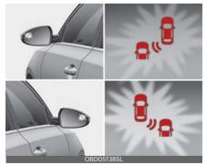
• To warn the driver a vehicle is detected, the warning light on the side view mirror will illuminate.
