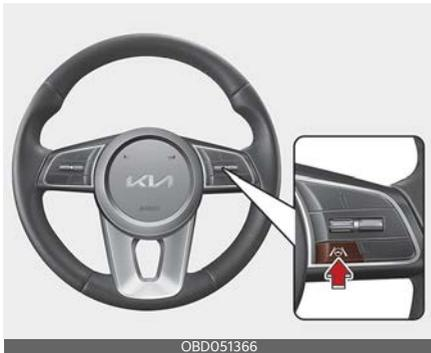
With the ignition switch or ENGINE START/STOP button in the ON position, press and hold the Lane Driving Assist button (
