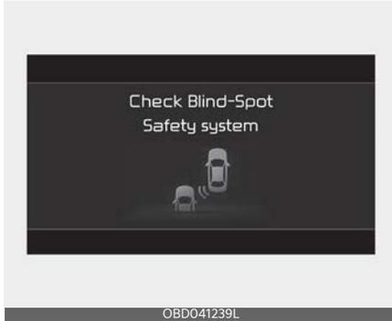
When Safe Exit Warning is not working properly, the 'Check Blind-Spot Safety system' warning message will appear on the cluster for several seconds, and the master (⚠️) warning light will illuminate on the cluster. In this case, have the vehicle inspected by an authorized Kia dealer.
