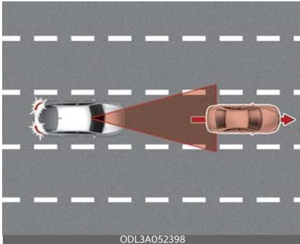
If the vehicle in front abruptly departs, Leading Vehicle Departure Alert may not operate properly.
