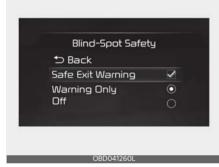
With the ignition switch or the ENGINE START/STOP button in the ON position, and select 'User Settings (LCD display) or Settings  $\rightarrow$  Vehicle (Infotainment System screen)  $\rightarrow$  Driver Assistance  $\rightarrow$ Blind-Spot Safety  $\rightarrow$  Safe Exit Warning' to turn on Safe Exit Warning and deselect to turn off the function.
