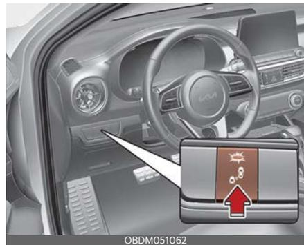
The indicator on the button will illuminate when Blind-Spot Safety button is pressed with the ignition switch or ENGINE START/STOP button in the ON position. If you press the button again, the button indicator and the function will be turned off. If the ignition switch or ENGINE START/STOP button is turned
