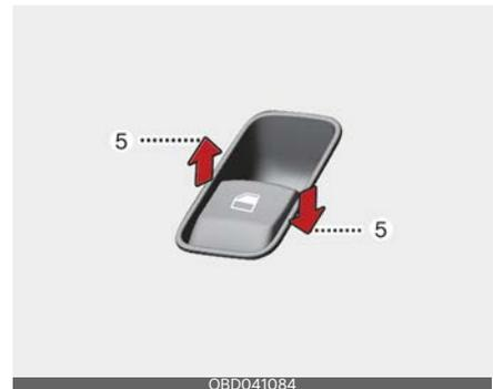
To open or close a window, press down or pull up the front portion of the corresponding switch to the first detent position (5).
