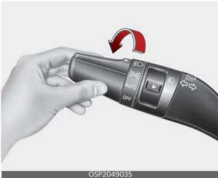
When the light switch is in the head light position, The head, tail, position, license and instrument panel lights will turn ON.
