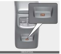
Plug the cable into the USB port, and charging will begin.
