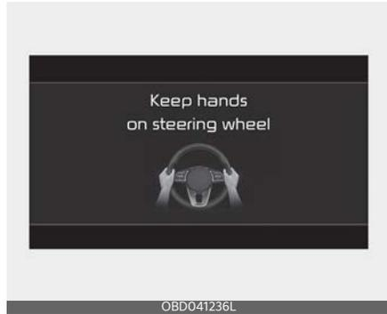
The hands-off warning appears when the function detects that the driver's hands are not on the steering wheel while Highway Driving Assist is in work.
