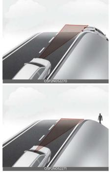
Forward Collision-Avoidance Assist may not detect other vehicles, pedestrians in front of you while driving uphill or downhill adversely affecting the performance of the sensors.
