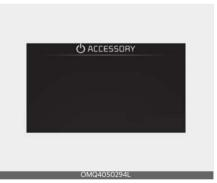
With Manual Transmission Press the ENGINE START/STOP button when the button is in the OFF position without depressing the clutch pedal.
