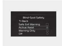
With the ignition switch or ENGINE START/STOP button in the ON position, select 'Driver Assistance  $\rightarrow$  Blind-Spot Safety' from the 'User Settings (LCD display) or Setup  $\rightarrow$  Vehicle (Infotainment System screen)' menu to set whether to use each function.
