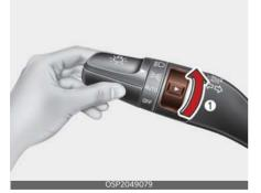
The fog lights will turn on when the fog light switch (1) is turned to the on position after the headlight is turned on. To turn off the fog lights:
