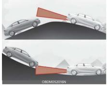
Blind-Spot Collision-Avoidance Assist may not operate properly when driving on a slope. The function may not detect the vehicle in the next lane or may incorrectly detect the ground or structure.
