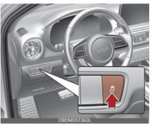
The Electronic Stability Control (ESC) system is designed to stabilize the vehi-
