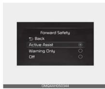
With the ignition switch or ENGINE START/STOP button in the ON position, select 'Driver Assistance  $\rightarrow$  Forward Safety' from the 'User Settings (LCD display) or Setup  $\rightarrow$  Vehicle (Infotainment System screen)' menu to set whether to use each function.
