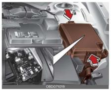
3. Check the removed fuse; replace it if it is blown. To remove or insert the fuse, use the fuse puller in the engine compartment fuse panel. 4. Push in a new fuse of the same rating, and make sure it fits tightly in the clips. If it fits loosely, consult an authorized Kia dealer.
