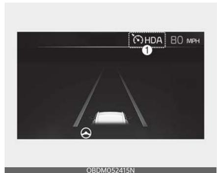
1. Highway Driving Assist indicator, whether there is a vehicle ahead and the selected distance level are displayed.
