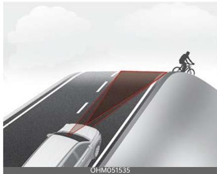
Forward Collision-Avoidance Assist may not detect other vehicle, pedes-
