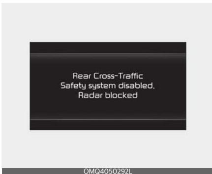
When the rear bumper around the rear-side radar or sensor is covered with foreign matters, such as snow or rain, or installing a trailer or carrier, it can reduce the detecting performance and temporarily limit or disable Rear Cross-Traffic Collision Warning.
