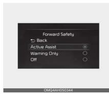
With the ignition switch or ENGINE START/STOP button in the ON position, select 'Driver Assistance  $\rightarrow$  Forward Safety' from the 'User Settings (LCD display) or Setup  $\rightarrow$  Vehicle (Infotainment
