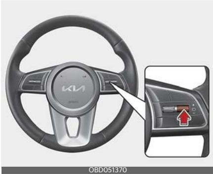
Press the ||⌚ switch to temporarily pause the set speed limit. The set speed limit will turn off but the Speed Limit indicator will stay on.
