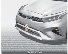
[1] : Front view camera, [2]: Front radar Refer to the picture above for the detailed location of the detecting sensors.
