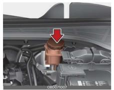
1. Before removing the reservoir cap and adding brake/clutch fluid, clean the area around the reservoir cap thoroughly to prevent brake/clutch fluid contamination.
