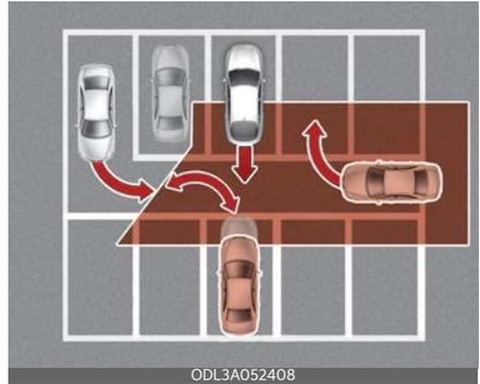
Rear Cross-Traffic Collision Warning may detect vehicles which are parking or pulling out near your vehicle (for example, a vehicle leaving beside your vehicle, a vehicle parking or pulling out in the rear area, a vehicle approaching your vehicle making a turn, etc.). If this occurs, the function may unnecessarily warn the driver.
