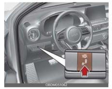
If you press the Blind-Spot Safety button while 'Warning Only' or 'Active Assist' selected the indicator on the button extinguishes and the function deactivates, and if you press the Blind-Spot Safety button while the function is off, indicator on the button illuminates and the function will operate as before it was turned off.
