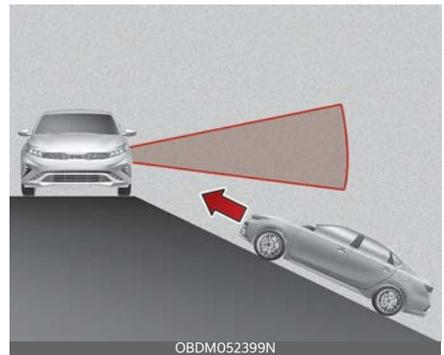
Rear Cross-Traffic Collision-Avoidance Assist may be limited when the vehicle is on an uphill or downhill slope, or near it, and may not detect the vehicle approaching from the left or right. If this occurs, the function may not warn the driver or control the brakes when necessary.
