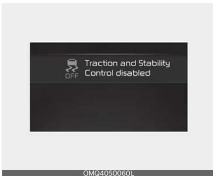
Press the ESC OFF button for more than 3 seconds. ESC OFF indicator light and message illuminates and ESC OFF warning chime will sound. At this state, the engine control function and brake control function does not operate. In other words, the vehicle
