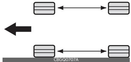
Rotate radial tires that have an asymmetric tread pattern only from front to rear and not from right to left.
