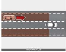
Blind-Spot Collision-Avoidance Assist helps detect and informs the driver that a vehicle is approaching at high speed from the blind spot area.
