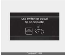
When Highway Driving Assist is operating, your vehicle will stop if the vehicle ahead of you stops. Also, if the vehicle ahead of you starts moving within 30 seconds after the stop, your vehicle will start as well. In addition, after the vehicle has stopped and 30 seconds have passed, the 'Use switch or pedal to accelerate' message will appear on the cluster. Depress the accelerator pedal or push the + switch, - switch or (|| ) switch to start driving.
