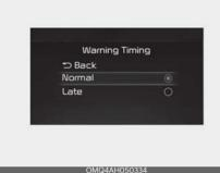
With the ignition switch or ENGINE START/STOP button in the ON position, select 'Driver Assistance  $\rightarrow$  Warning Timing' from the 'User Settings (LCD display) or Setup  $\rightarrow$  Vehicle (Infotainment System screen)' menu to change the initial warning activation time for Forward Collision-Avoidance Assist.
