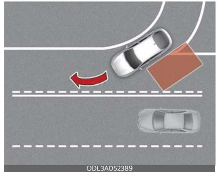
Blind-Spot Collision Warning may not operate properly when driving where the road merges or divides. The function may not detect the vehicle in the next lane.
