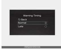
With the ignition switch or ENGINE START/STOP button in the ON position, select 'Driver Assistance  $\rightarrow$  Warning Timing' from the 'User Settings (LCD display) or Setup  $\rightarrow$  Vehicle (Infotainment System screen)' menu to change the initial warning activation time for Forward Collision-Avoidance Assist.
