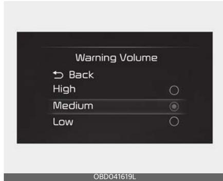
With the ignition switch or ENGINE START/STOP button in the ON position, select 'Driver Assistance → Warning Volume' from the 'User Settings (LCD display) or Setup → Vehicle (Infotainment System screen)' menu to change the Warning Volume to 'High', 'Medium' or 'Low' for Forward Collision-Avoidance Assist.
