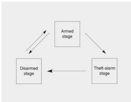
This system is operated in three stages: the first is the "Armed" stage, the second is the "Theft-alarm" stage, and the third is the "Disarmed" stage. If triggered, the system provides an audible alarm with blinking of the hazard warning lights.
