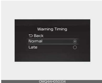
With the ignition switch or ENGINE START/STOP button in the ON position, select 'Driver Assistance → Warning Timing' from the 'User Settings (LCD display) or Setup → Vehicle (Infotainment System screen)' menu to change the initial warning activation time for Forward Collision-Avoidance Assist.
