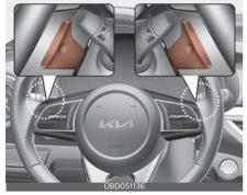
The paddle shifter is available when the shifter lever is the D (Drive) position or the manual mode.
