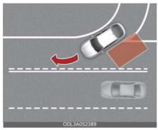
Blind-Spot Collision-Avoidance Assist may not operate properly when driving where the road merges or divides. The function may not detect the vehicle in the next lane.Always pay attention to road and driving conditions while driving.
