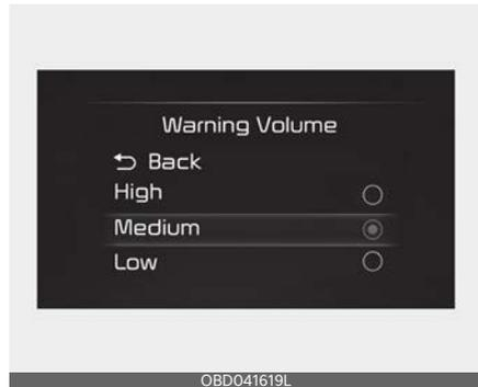
With the ignition switch or the ENGINE START/STOP button in the ON position, select 'Driver Assistance → Warning Volume' from the Settings menu to change the Warning Volume to 'High', 'Medium' or 'Low' for Reverse Parking Distance Warning.
