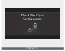
When Blind-Spot Collision Warning is not working properly, the 'Check Blind-Spot Safety system' warning message will appear on the cluster, and the function will turn off automatically, or the function will be limited. In this case, have your vehicle inspected by an authorized Kia dealer.
