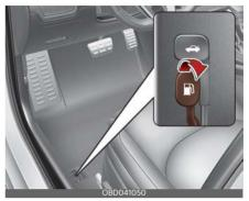
The fuel-filler door must be opened from inside the vehicle by pulling up on the fuel-filler door opener located on the front floor area on the driver's seat.
