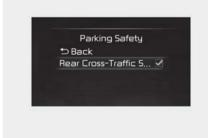
With the ignition switch or ENGINE START/STOP button in the ON position, select 'Driver Assistance  $\rightarrow$  Parking Safety  $\rightarrow$  Rear Cross-Traffic Safety' from the 'User Settings (LCD display) or Setup  $\rightarrow$  Vehicle (Infotainment System screen)' menu to turn on Rear Cross-Traffic Collision Warning and deselect to turn off the function.
