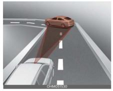
Your vehicle speed can be reduced due to a vehicle in the adjacent lane. Apply the accelerator pedal and select the appropriate set speed. Check to be
