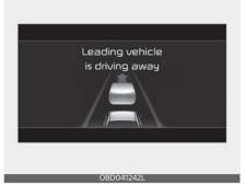
When a detected vehicle in front departs from a stop, Leading Vehicle Departure Alert will inform the driver by displaying the 'Leading vehicle is driving away' message on the cluster and an audible warning will sound.
