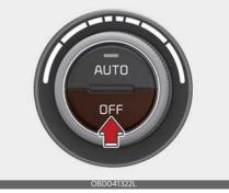
Press the OFF button to turn off the air climate control system. However, you can still operate the mode and air intake buttons as long as the ignition switch or the ENGINE START/STOP button is in the ON position.
