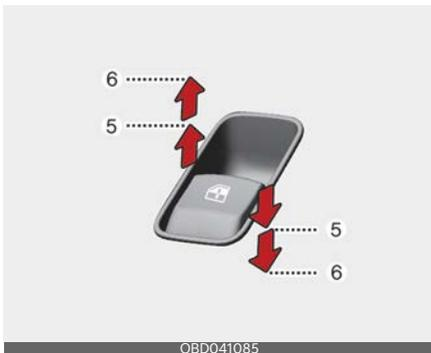
Pressing or pulling up the power window switch momentarily to the second detent position (6) completely lowers or raises the window even when the switch is released. To stop the window at the desired position while the window is in
