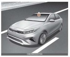
[1]: Front view camera Refer to the picture above for the detailed location of the detecting sensors.
