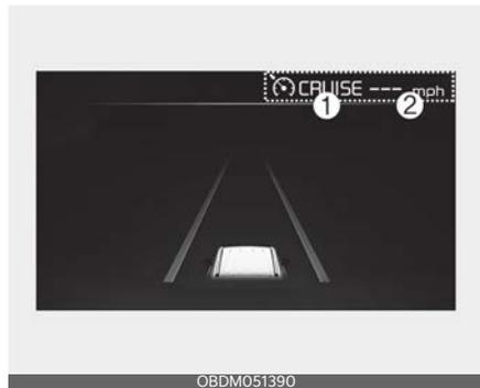
You can see the status of Smart Cruise Control operation in the Driving Assist view on the cluster. Refer to "Instrument cluster" on page 4-53.
