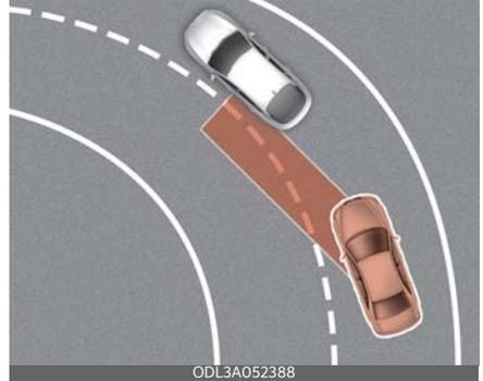
Blind-Spot Collision Warning may not operate properly when driving on the curved road. The function may recognize the vehicle in the same lane. Always pay attention to road and driving conditions while driving.
