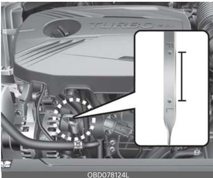
3. Turn the engine off, remove the oil filler cap and pull the dipstick out. Wait for 15 minutes for the oil to return to the oil pan.
