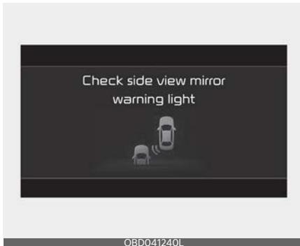
When the outside rear view mirror warning light is not working properly, the 'Check side view mirror warning light' warning message will appear on the cluster for several seconds, and the master (⚠️) warning light will appear on
