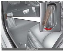
Open the hood after turning off the engine on a flat surface, shifting the shift lever to the P (Park, for Dual Clutch Transmission/ Intelligent Variable Transmission) or first gear or R (Reverse, for Manual Transmission) and set the parking brake.
