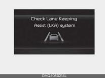
When Lane Keeping Assist is not working properly, the 'Check Lane Keeping Assist (LKA) system', warning message will appear and the yellow ( ) indicator light will illuminate on the cluster. In this case, have the function inspected by an authorized Kia dealer.
