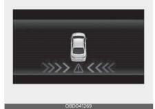
To warn the driver of an approaching vehicle from the rear left/right side of your vehicle, the side view mirror will blink and a warning will appear on the cluster. At the same time, an audible warning will sound. If Rear View Monitor is operating, a warning will also appear on the infotainment screen.
