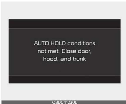
At this moment, press the [AUTO HOLD] button after closing the driver's door, engine hood and trunk.
