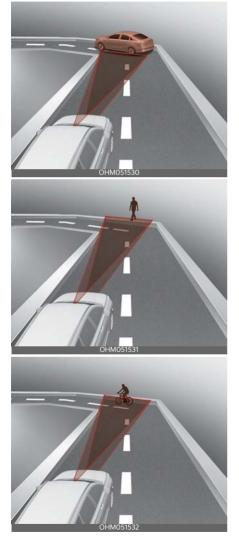
Forward Collision-Avoidance Assist may detect a vehicle or pedestrian in the next lane or outside the lane when
