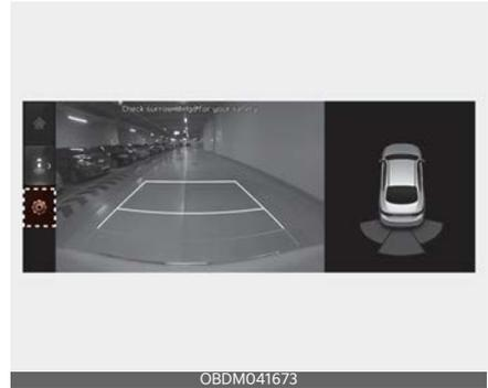
You can change Rear View Monitor 'Display Contents' of 'Display Settings' by touching the setup icon (⚙️) on the screen while Rear View Monitor is operating, or selecting 'Setup → Vehicle → Driver Assistance → Parking Safety → Camera Settings' from the Infotainment System screen while the engine is on.
