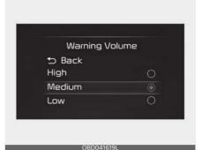
With the ignition switch or ENGINE START/STOP button in the ON position, select 'Driver Assistance  $\rightarrow$  Warning Volume' from the 'User Settings (LCD display) or Setup  $\rightarrow$  Vehicle (Infotainment System screen)' to change the Warning Volume to 'High', 'Medium', 'Low' for Blind-Spot Collision Warning.
