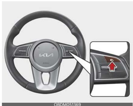
Press the Driving Assist button to turn Cruise Control off. The Cruise indicator will go off.
