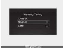
With the ignition switch or ENGINE START/STOP button in the ON position, select 'Driver Assistance → Warning Timing' from the 'User Settings (LCD display) or Setup  $\rightarrow$  Vehicle (Infotainment System screen)' menu to change the initial warning activation time for Rear Cross-Traffic Collision-Avoidance Assist. When the vehicle is first delivered, warning timing is set to Normal. If you change the Warning Timing, the Warning Timing of other Driver Assist systems may change.
