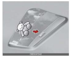
If the sunroof glass senses any obstacle while it is closing automatically, it will reverse direction then stop at a certain position. The auto reverse function may not work if an object thin or soft is caught between the sliding sunroof glass and sunroof sash.
