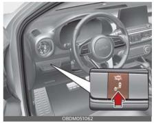
The indicator on the button will illuminate when Blind-Spot Safety button is pressed with the ignition switch or ENGINE START/STOP button in the ON position. If you press the button again, the button indicator and the function will be turned off. If the ignition switch or ENGINE START/STOP button is turned OFF and ON, the function returns to the previous state. When the function is not being used, turn the function off by pressing the button.
