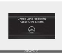
When Lane Following Assist is not working properly, the 'Check Lane Following Assist (LFA) system' warning message will appear on the cluster (turns off after a certain time) and the /! warning light will illuminate. In this case, have the function checked by an authorized Kia dealer.
