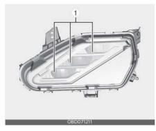
If the front fog lamp (LED) (1), does not operate, have the vehicle checked by an authorized Kia dealer. The LED lamps cannot be replaced as a single unit because it is an integrated unit. The LED lamps has to be replaced with the unit.A skilled technician should check or repair the front fog lamp (LED), for it may damage related parts of the vehicle.
