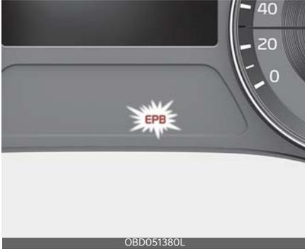
If the EPB malfunction indicator remains on, it indicates that the EPB may have malfunctioned. If this occurs, have the system checked by an authorized Kia dealer.
