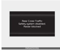
When the rear bumper around the rearside radar or sensor is covered with foreign matters, such as snow or rain, or installing a trailer or carrier, it can reduce the detecting performance and temporarily limit or disable Rear Cross-Traffic Collision Warning. If this occurs, the 'Rear Cross-Traffic Safety disabled. Radar blocked' warning message will appear on the cluster.
