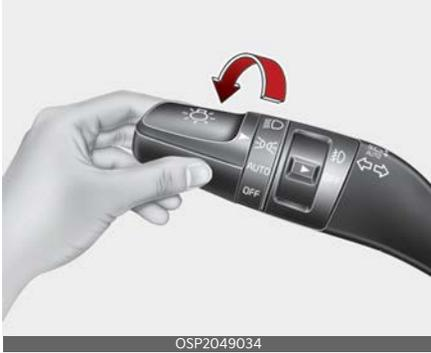
When the light switch is in the position lamp position, the front position lamp and, tail, license light will turn ON.
