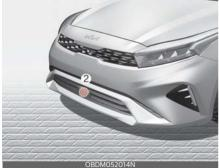
[1]: Front view camera, [2]: Front radar The front view camera and front radar are used as a detecting sensor to detect vehicles in front. Refer to the picture above for the detailed location of the detecting sensor.
