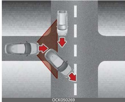
When a vehicle ahead disappears at an intersection, your vehicle may accelerate. Always pay attention to road and driving conditions while driving.
