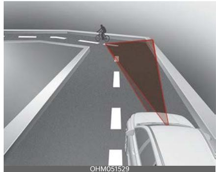
The front view camera or radar sensor recognition function may not detect the vehicle, pedestrian or cyclist traveling in front on a curved road.
