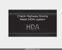
When Highway Driving Assist is not working properly, the 'Check Highway Driving Assist (HDA) system' warning
