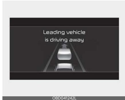
When a detected vehicle in front departs from a stop, Leading Vehicle Departure Alert will inform the driver by displaying the 'Leading vehicle is driving away' message on the cluster and an audible warning will sound.
