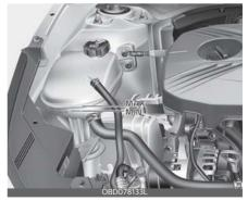
Check the condition and connections of all cooling system hoses and heater hoses. Replace any swollen or deteriorated hoses.
