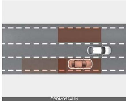
Blind-Spot Collision Warning helps detect and informs the driver that a vehicle is in the blind spot.
