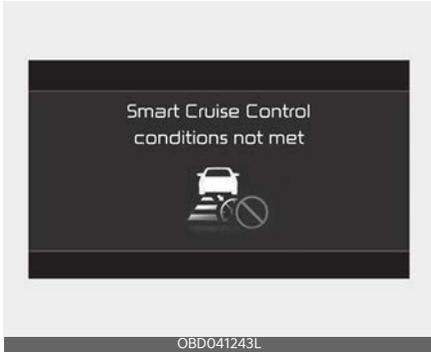
If the Driving Assist button, +, - or || ↻ switch is operated when Smart Cruise Control's operating conditions are not satisfied, the 'Smart Cruise Control conditions not met' will appear on the cluster, and an audible warning will sound.
