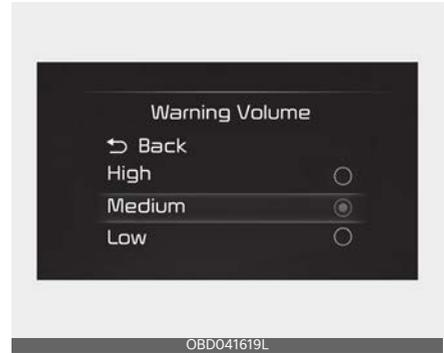
With the ignition switch or ENGINE START/STOP button in the ON position, select 'Driver Assistance → Warning Volume' from the 'User Settings (LCD display) or Setup → Vehicle (Infotainment System screen)' to change the Warning Volume to 'High', 'Medium', 'Low' for Blind-Spot Collision Warning.
