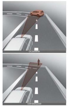
Forward Collision-Avoidance Assist may detect a vehicle or pedestrian in the next lane or outside the lane when driving on a curved road.
