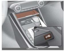
Firmly close all doors, and the ignition switch or ENGINE START/STOP button is ON. To start wireless charging, place the smart phone equipped with wireless charging function on the wireless charging pad.
