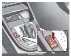
The temperature setting of the seat changes according to the button position.
