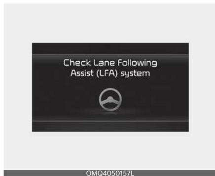
When Lane Following Assist is not working properly, the 'Check Lane Following Assist (LFA) system' warning message will appear on the cluster (turns off after a certain time) and the
