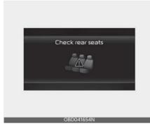
You can activate or deactivate the Rear Occupant Alert by selecting 'User Settings (LCD display) or Settings  $\rightarrow$  Vehicle (Infotainment System screen)  $\rightarrow$  Convenience  $\rightarrow$  Rear Occupant Alert'.
