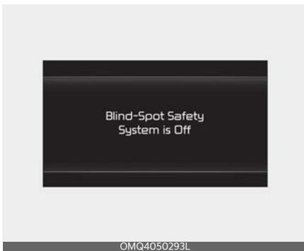
When the engine is restarted with Blind-Spot Collision Warning off, the 'Blind-Spot Safety System is Off' message will appear on the cluster.
