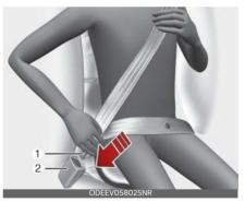
• Pull it out of the retractor and insert the metal tab (1) into the buckle (2). There will be an audible "click" when the tab locks into the buckle.
