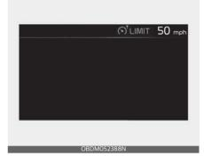
3. The set speed limit will be displayed on the cluster. If you would like to drive over the preset speed limit, depress the accelerator pedal beyond the pressure point to activate the kickdown function.
