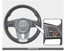
Press the [] ) switch to temporarily pause the set speed limit. The set speed limit will turn off but the Speed Limit indicator will stay on.
